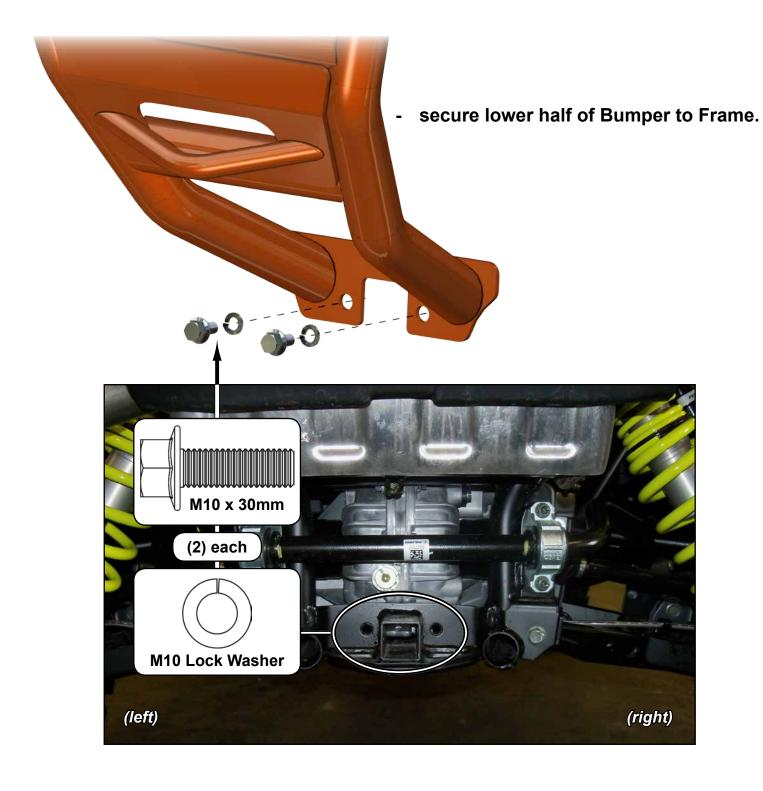
Align to machine and tighten hardware completely.
