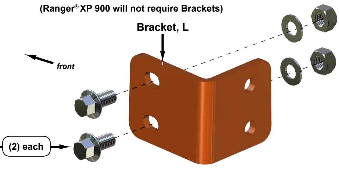
Ranger® XP 900: Install directly to Cab Frame with hardware shown.
