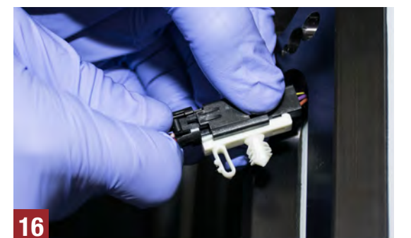
Fig. 16 Re-connect the light housing in the reverse manner as removal. With the power harness attached, route back through the opening and with the clips aligned with the small openings push up to attach back in place. Fig. 17-19 Re-install the light housing utilizing the provided longer button head cap screws for the middle two (2) holes and the shorter button head cap screws for the outer two (2) holes. With the 3rd Brake Light Antenna Adapter installed, attach desired compatible antenna with NMO standard threaded antenna connector and fasten the PL-259 male UHF connector to preferred 2-way radio.
