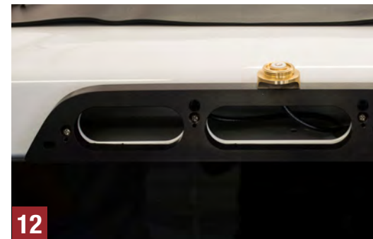
Fig. 8 Route the antenna cable into the cab following the brake light harness. From inside the cab, access the cable and route to final desired location. Fig. 9-12 To attach the antenna adapter, align and attach the adapter utilizing the four (4) factory mounting holes and the provided phillips pan head screws. Fig. 13-15 With the adapter in place, attach the support bracket by drilling two (2) 3/16" holes through the top middle holes of the adapter. Next, feed the support bracket into the opening and align with drilled holes. Using the provided socket head cap screws secure in place.
