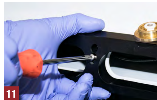
Fig. 8 Route the antenna cable into the cab following the brake light harness. From inside the cab, access the cable and route to final desired location. Fig. 9-12 To attach the antenna adapter, align and attach the adapter utilizing the four (4) factory mounting holes and the provided phillips pan head screws. Fig. 13-15 With the adapter in place, attach the support bracket by drilling two (2) 3/16" holes through the top middle holes of the adapter. Next, feed the support bracket into the opening and align with drilled holes. Using the provided socket head cap screws secure in place.
