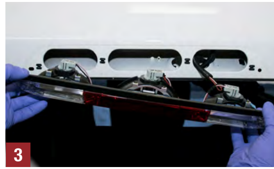
Fig. 2-3 Using a 9/32" (7mm) nut driver remove the four (4) screws holding the housing in place and pull away from the cab. Fig. 4-7 Disconnect the light housing at the pigtail connector not at the light. Access the connector by pushing down on the clips and pulling through the opening on the right. Disconnect by pressing down on the retaining clip, then slide away from each other. Place the removed housing in a safe location to be re-installed later.
