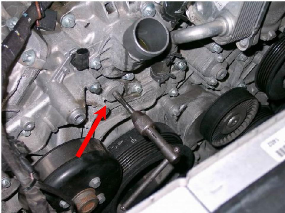
A M8 tread has to be made in the O.E. water pump to fit the Kleemann bracket, use the long M 8 torx bolt from the O.E. pulley wheel in the other side.
