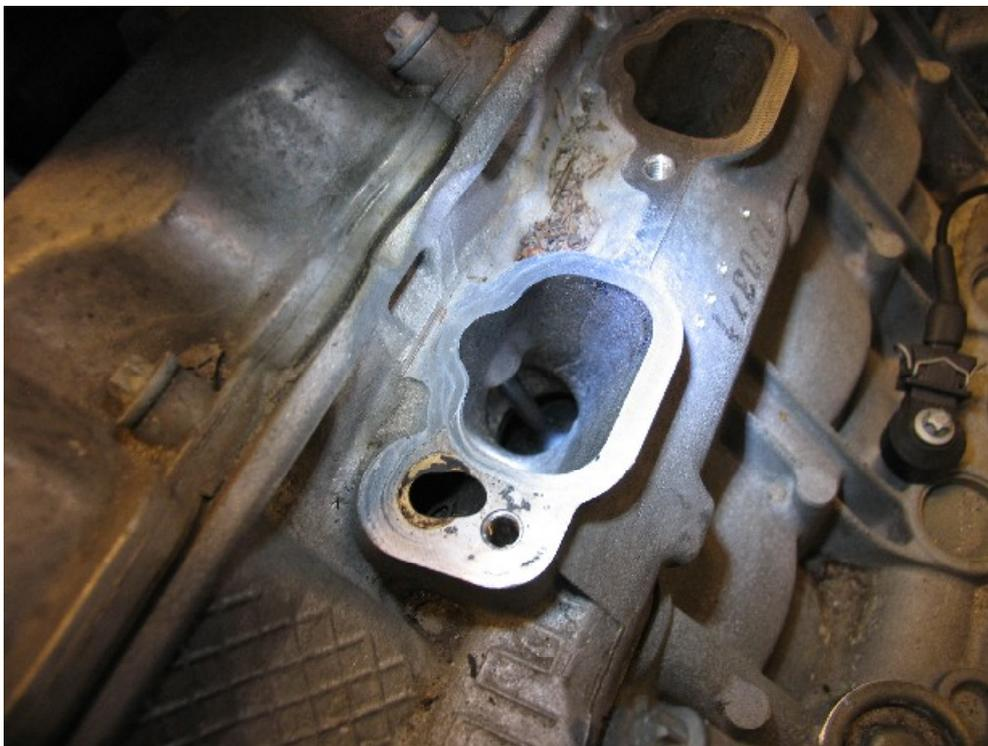
make sure that nothing have entered the ducts, like some of the screws from the O.E. manifold
