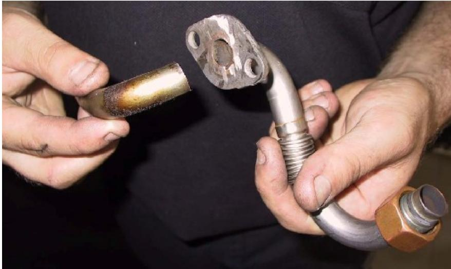
Install the EGR pipe on the KLEEMANN manifold. Use the original screws and gasket. **Apply Loctite 243 on the screws.**
