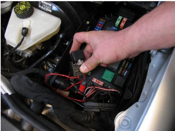
A wire is drawn from the pump+ to the relay box where it is joined in the kit relay as shown.
