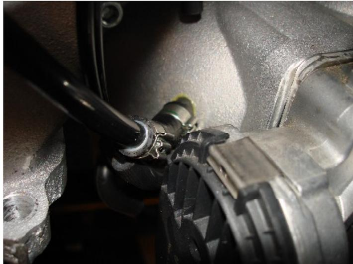
Connect the supplied hose to the 8mm pipe on the inlet housing using the supplied cobra clamps, in order to connect the tank ventilation. Next to the 8 mm tap there is two 4 mm taps. Mount the vacuum line so that it is long enough to reach the front of the compressor.
