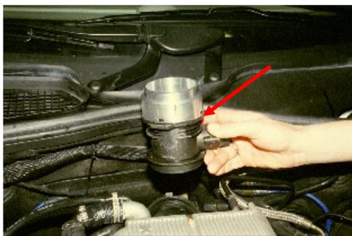
Install the original 90 degree intake hose on the throttle body.
