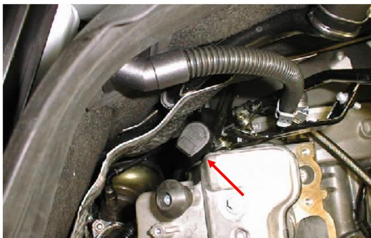
Move the automatic transmission oil dipstick as shown in the picture.
