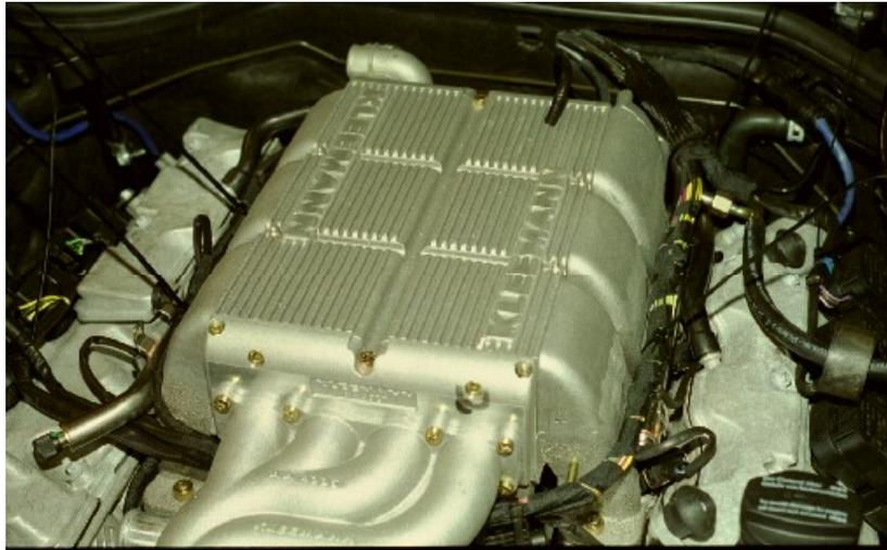
Re-route the engine wiring harness so that it passes under the water manifold. Reconnect all plugs to their original locations. Use zip ties to secure the engine wiring harness to the fuel rail.
