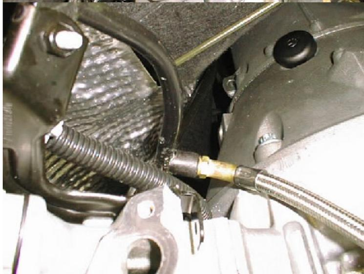
The oil pin is placed different on the C W203.
