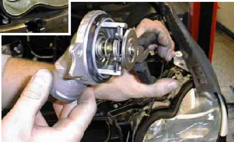
On the SLK you have to use the O.E thermostat housing and rotate it so it clears the SC and fit bigger washers to the screws. Note that the screws do not fit the holes anymore but are lined up against the edge of the holes which is why we recommend bigger washers.
