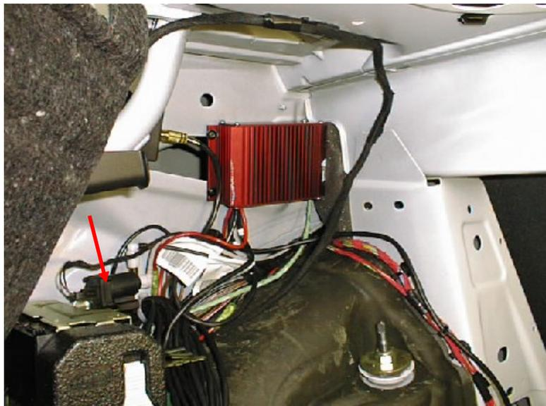
The C W203 has an in-tank centerfugal fuel pump. This pump is not able deliver enough pressure for proper fuel mixtures for full boost at high engine speeds. The pump booster gives the fuel pump 17VDC when boost pressure is present.
