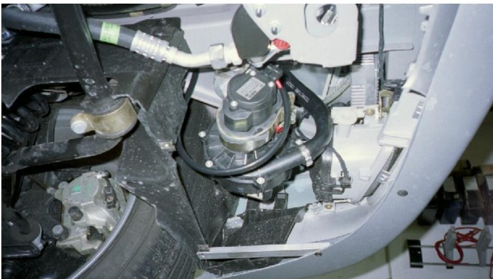
Install the air pump where space is available. Due to different equipment available on different vehicles a definitive location cannot be suggested.
