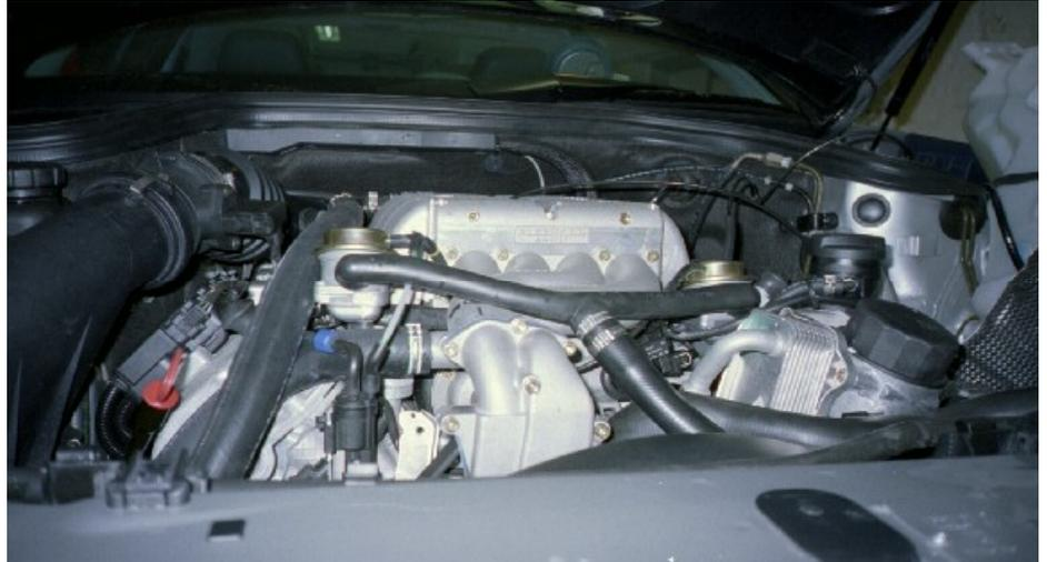
Grind the aluminum housing of the dash pots so they fit back onto the KLEEMANN intake manifold.
