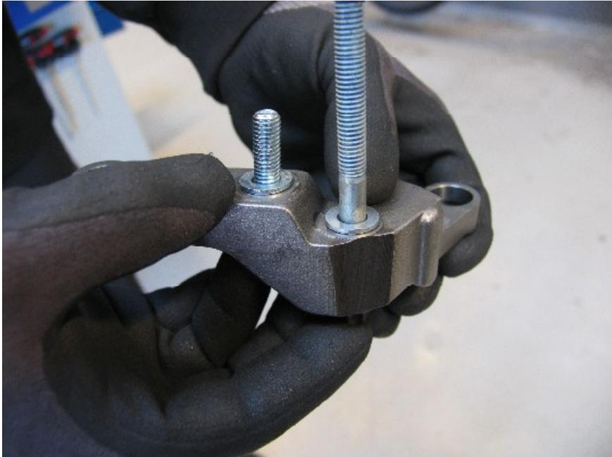
Fit 2 washers on to the support pulley in order to make it fit the motor block
