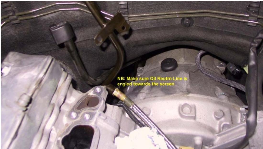
Dismount the alternator and the oil dipstick tube. Install the new KLEEMANN dipstick tube. Reinstall the alternator. Remember to have a bucket under the car so that the oil from removing the dipstick tube is collected.
