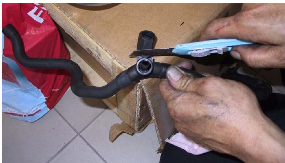
Cut off the breather hose as shown, and install it onto the throttle body.
