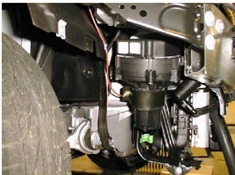
Mount the auxiliary air pump behind the valence panel and behind the driving light right side.
