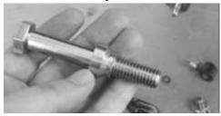
12. Insert the new  $\frac{1}{2}$  x 3  $\frac{1}{4}$ " hex bolt. Slide the bolt through the alignment bushing, then the heim joint and then through another alignment bushing. Insert the bolt through the knuckle assembly.
