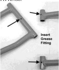
6. Now reinstall the bushings, sleeves, and ball joints into the new arms. If you place some grease on them it makes the installations easier.
