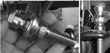
13. Place the ½" washer and ½" lock nut on the bolt and torque tight.
