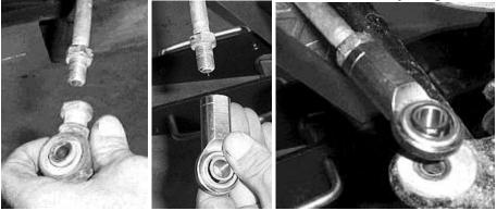
10. To connect the new heim joint to the knuckle assembly you will need to use a ½" drill bit and drill a larger hole where the tie rod connects to the knuckle.
