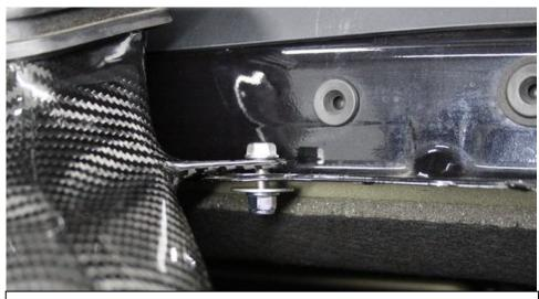
22. Insert the 2 screws through the mounts on the top rear of the duct and through the stock mounting locations. We removed the rubber grommets from these holes in step 7. Do not tighten yet.
