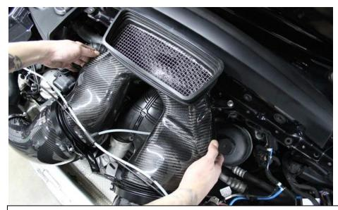
30. You will need some help for this step – the duct needs to be pulled forwards so that the rubber seals compress onto the filter housings.
