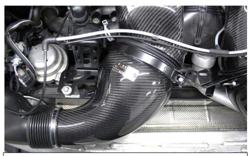
28. Repeat this process for the other side. Once lined up, secure the large filter clamp and the hose clamp around the stock inlet pipe.
