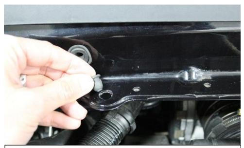
7. Remove the 2 rubber grommets which the duct was pushed into.
