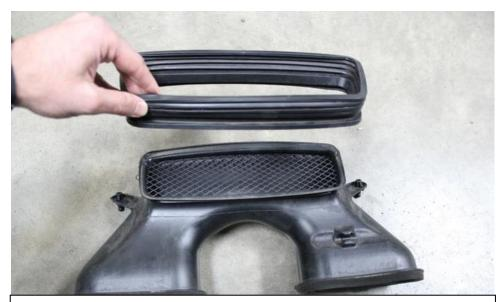
8. Remove the rubber surround from the top of the duct. We will use this later.
