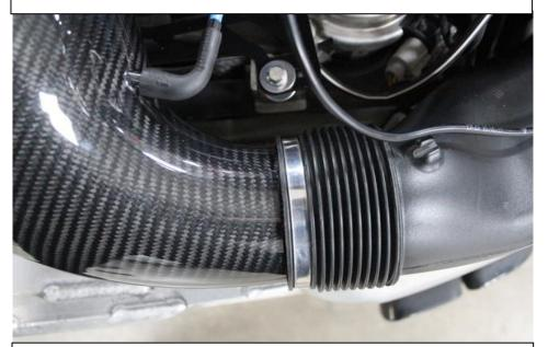
27. Now tighten the hose clamp at the stock inlet pipe.
