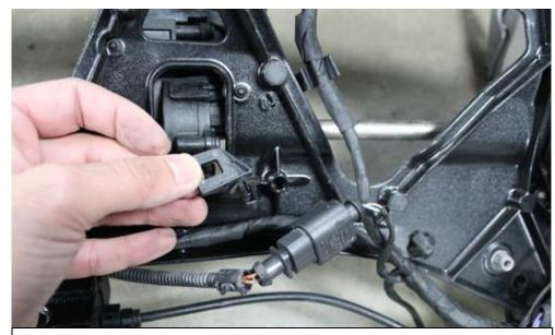
34. With the connector unclipped, remove the bracket for the connector from the frame.
