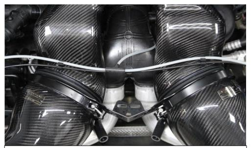
32. The fully secured system should now have a good seal between the duct and the filter housings.
