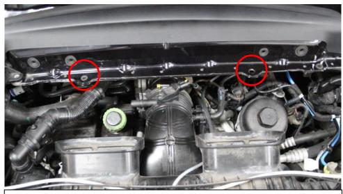
6. Remove the intake duct by simply pulling it upwards. It is held in place with rubber grommets which are circled above.
