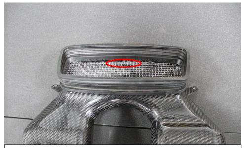
19. The rubber surround should secure around the rim at the top of the new duct. Logo on the mesh should be positioned as indicated by the circle.
