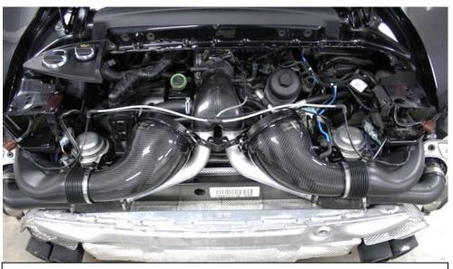
10. Take the filter housing assembly and position the brackets on top of the stock airbox mounts. Push the stock inlet tubes onto each intake housing. Don't tighten yet.
