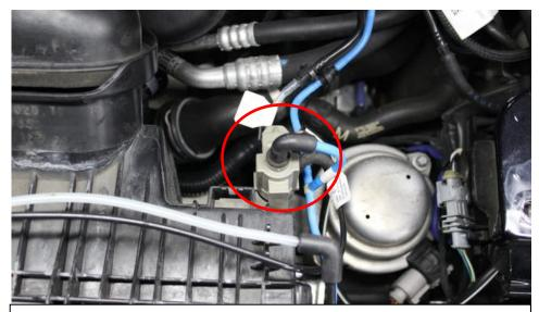
4. Remove the module on the right side of the airbox.
