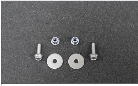
21. Take the remaining shorter M6 screws with 2 washers and lock nuts.
