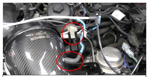
12. Push the right side module onto the bracket and push the vacuum connector into the outlet on the filter housing.
