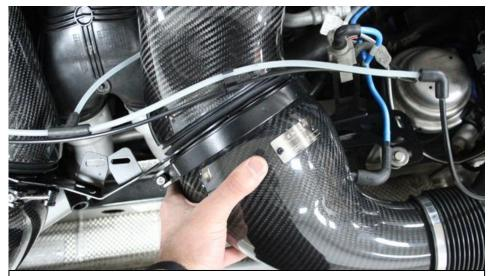
25. Start with one side and rotate the housing so that it sits square with the duct. As you rotate, the angle of the housing will change with respect to the duct. The rubber seal should be in full contact all the way around the face of the filter housing. If required – move the entire filter housing assembly left or right to centralise it with the duct.
