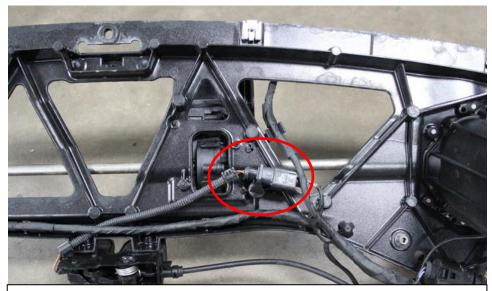
33. For extra clearance – unclip the connector from the underside of the metal frame which holds the spoiler motors.
