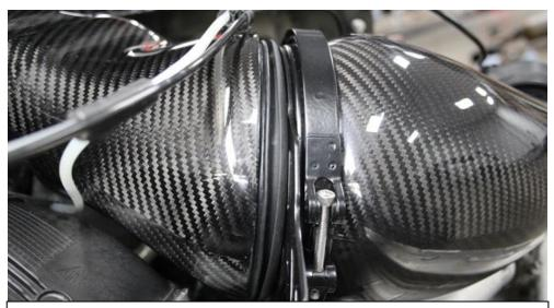
26. Once fully sealed as shown, tighten the large clamp around the housing.
