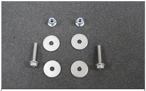
14 Take the 2 longer M6 screws from the pack along with 4 washers and 2 lock nuts.
