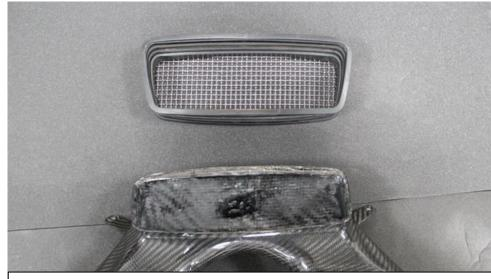
18. Take the carbon duct and now push the rubber surround with mech into the top of the new duct.
