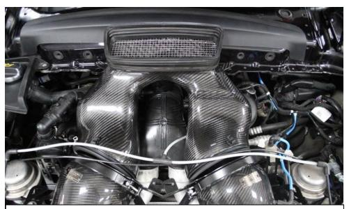
20. Now place the duct on top of the filter housings. We will now line up the housings to the duct.
