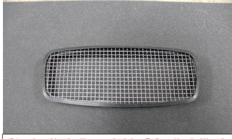
17. Insert the mesh into the rubber surround at the base. The Eventuri logo should be at the top (not shown here). Back of the rubber surround shown above.
