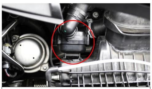
3. Remove the module at the rear of the airbox located on the left side. There is a clip in the airbox which needs to be depressed to release this module.
