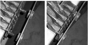
8. Next using the two large spacers and 6mm x 130mm bolts connect the fan to the brackets. Secure them using <sup>1</sup>/<sub>4</sub>" flat washer and 6mm lock nuts. Place a 1/4" washer on the bolt, push it through the connecting point of the frame. Next place a spacer on the bolt, then slide the bolt through the fan and secure it with a <sup>1</sup>/<sub>4</sub>" washer and 6mm lock nut.
