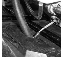
25. Using the remaining <sup>1</sup>/<sub>4</sub>" black hose provided in the kit, run the overflow hose from top of the over flow bottle, down through the other hole that was drilled in the access panel.
