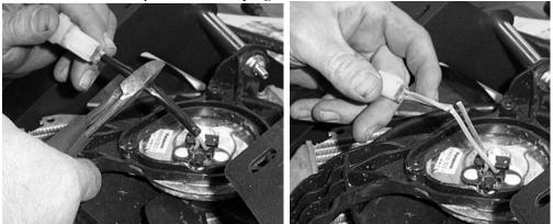
14. Using the butt connecters and wire provided, extend the fan plug. Attach the green to green and blue to blue.
