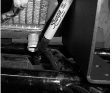
17. Drill the hole in the plastic, it needs to be 1" in diameter.
