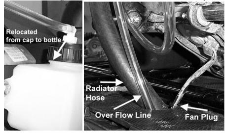
26. Now connect the inlet and outlet hoses to the hoses you left connect to the engine. Secure the hoses to the fitting with the clamps provided in the kit.
