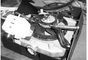
12. Next you will need to extend the fan wires on the back of the fan.
