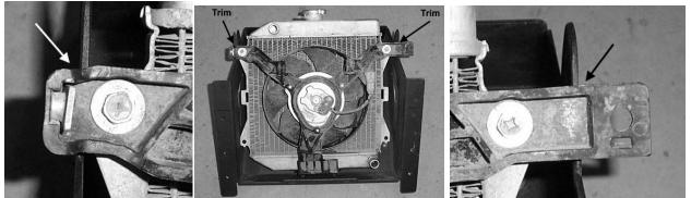
7. Once the grommets are installed and the fan has been trimmed, insert the bottom of the radiator into the grommets.
