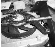
9. Now connect the bottle and bottle bracket to the right leg using two <sup>1</sup>/<sub>4</sub>" x <sup>3</sup>/<sub>4</sub>" carriage bolts, two <sup>1</sup>/<sub>4</sub>" x <sup>3</sup>/<sub>4</sub>" hex bolts, two <sup>1</sup>/<sub>4</sub>" washers and four <sup>1</sup>/<sub>4</sub>" lock nuts.
