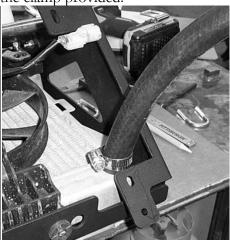
19. You need to insert the hose through the hole you drilled in the plastic as you are installing the radiator relocation kit to the rack.
