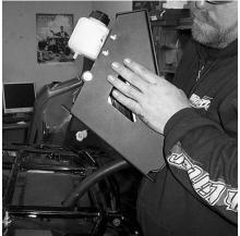
20. Connect the radiator to the rack using the <sup>1</sup>/<sub>4</sub> x 1" bolts, U-bolts, <sup>1</sup>/<sub>4</sub>" washers and <sup>1</sup>/<sub>4</sub>" lock nuts provided in the kit.
