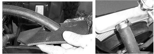
24. Push fan wire through the access panel and attach the access panel to the ATV.
