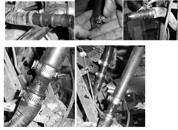
27. **VERY IMPORTANT:** Place the protective sleeve around the hoses to keep them from rubbing on the rack and plastic fenders. If the hose is left unprotected the vibration of the hose against the rack and fenders will cause a hole to form in the hose.
