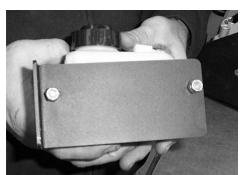
11. Now, connect the plate to the right leg. Using the <sup>1</sup>/<sub>4</sub>" x <sup>3</sup>/<sub>4</sub>" carriage bolts connect the plate and secure it with the <sup>1</sup>/<sub>4</sub>" lock nuts.
