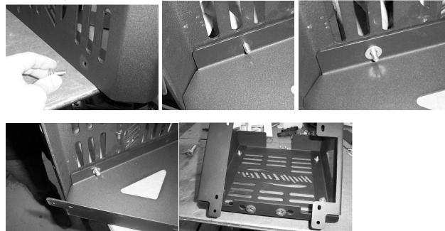
5. Where the bottom of the stock radiator attaches to the frame there are two rubber grommets that you will need to place in the two center holes at the base of the new face plate. Once they are installed insert the bottom of the radiator into the grommets.
