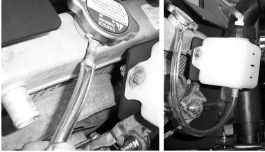
23. Now run two feet of hose through the access panel, placing a clamp on the end that will connect to the radiator. Connect the hose to the radiator.
