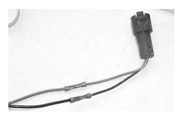
16. Wrap the wires in black tape, and run it through the ½" wire loom. Connect the end back to the connector under the plastic,
