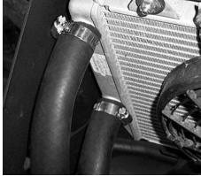
9. Connect the hoses using the 1" 90° fitting and 1" straight fitting. The straight fitting connect to the hose on the lower hose that runs from the thermostat and the 90° fitting goes on the hose that runs from the lower right side to the inlet on the upper part of the radiator.
