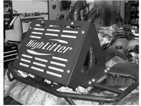
21. Fill the radiator and overflow bottle with factory approved fluid. Make sure that all air is removed from the system.
