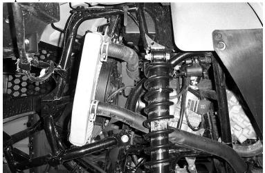
2. Remove the stock radiator and unplug the fan from the ATV.
