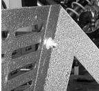
5. The bottom of the stock radiator has two rubber grommets that you will need to place in the holes at the base of the new face plate. They may still be attached to the frame and did not come out when you removed the radiator.
