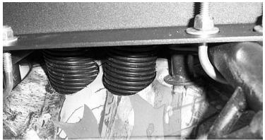
19. Connect the radiator to the rack using the U-bolts, 1/4" washers and 1/4" lock nuts provided in the kit.
