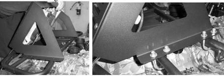
Note: On the left side of the rack you will drill two openings, one for the inlet hose and one for the outlet hose. On the right side you drill a hole using a  $1\frac{1}{2}$  hole saw for the over flow bottle intake and vent lines and the fan wires.
