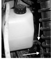
12. Connect to the overflow line located on the lower portion of the bottle a ¼" hose barb. Then connect the 3/16" hose provided in the kit to the barb and run line up to the port on the filler neck.
