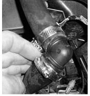
11. Run the vent line and overflow line from the overflow bottle up to the open hole in the plastic
