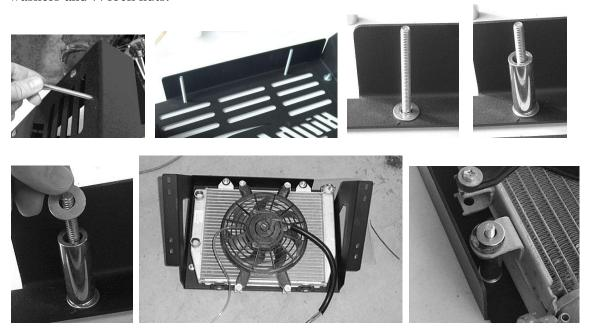
7. Once the kit is assembled, place the kit on the front rack and temporarily mount it to the rack using the U-bolts provided in the kit. Next mark the holes that need to be drilled to allow the hoses and wires for the fan to pass through the plastic and rack. Mark all holes and remove the radiator kit from the rack. Drill the holes using 1 3/4" hole saw.
