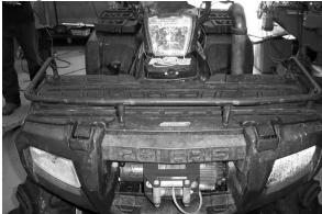
6. Preassemble the new radiator relocating kit. Assemble the frame using the ½ x ¾ carriage bolts (4ea), ¼ lock nuts (4ea), and ¼ flat washers (4ea).
