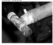
17. Run the hoses from kit to the inlet and outlet hoses that are still attached to the engine. You will need to cut to length. Using the clamps provided in the kit connect the hoses to the inlet and outlet ports on the radiator. You will join the new hoses to the old hoses you left attached to the engine using the fittings and clamps provided in the kit.
