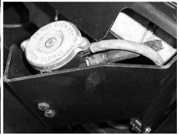
12. Once the kit is assembled, place the kit on the front rack and mark the holes that need to be drilled to allow the hoses and wires for the fan will pass through the rack.
