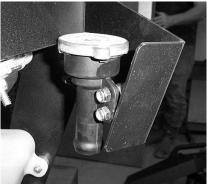
11. Attach the hoses from the neck to the radiator and from the neck to the overflow bottle. You will need to reuse the small OE clamps to hold the hose in place from the neck to the radiator. The small black hose is provided, but you will need to cut the overflow line.
