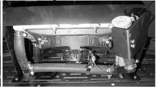
21. Insert 90° fittings into the hoses under the radiator and lid. Now connect hose to the 90° fittings and run them down to the stock hoses still connected to the engine.
