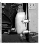
10. Next attach the filler neck and radiator cap to the top of the right leg of the rack mount kit. Use two of the medium spacers, ½ x 2 ½ bolts and ½ lock nuts.
