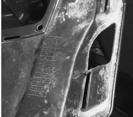
10. Next you will need to trim a small area near where the right side of the front rack connects to the ATV. You will run the fan wires up through this area and up by the front rack.
