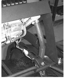
20. On the older model Grizzlies there is an extra ¼" bung on the radiator. We provide enough black hose for you to run a new line from the new relocated position to the cylinder head. This is only on the older model radiators that have this extra bung.
