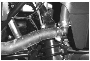
13. Now run the hoses up through the two holes you cut in the vented plastic on the top rack.
