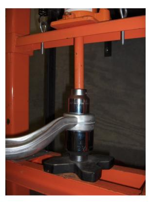
Press out stock bushing using appropriate bushing press and driver.
