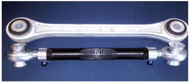
Try to match length of new link to that of old, center to center of the bores.
