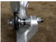
It is also important to ensure the endlinks have good articulation in another direction of motion – the twisting motion, as seen below:
