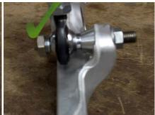
As a rule, you want the endlink to be as close to vertical as possible. If the bearing is not installed with sufficient articulation angle, then under suspension travel the endlink will bind. To obtain good articulation, use the extra ring spacers supplied to adjust the position of the ball joint at the lower arm to best match the alignment to the installation hole on the sway bar:
