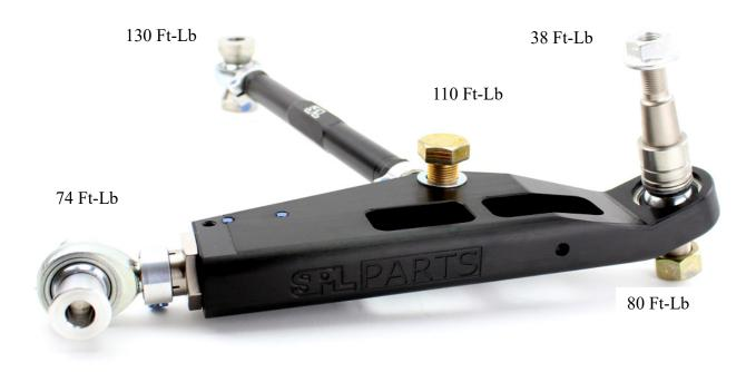
The picture above lists the torque specs. **DO NOT OVERTORQUE!** \*SPL Parts is not liable for any issues due to overtorque.\*
