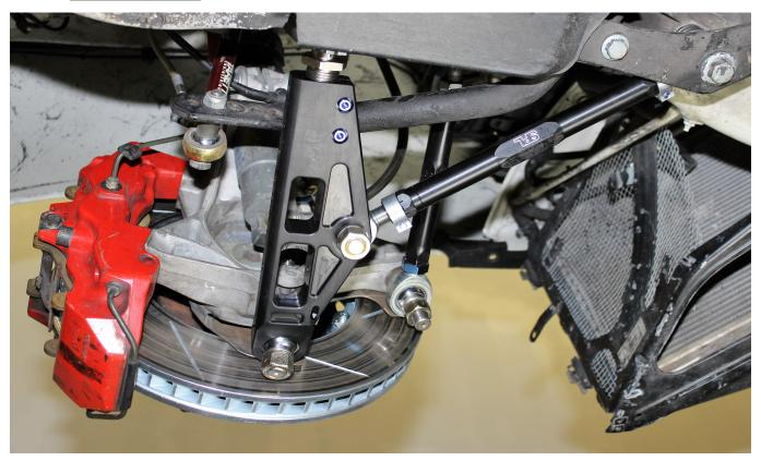
This picture shows the track arm with 2 spacers for anti dive installed, as well as spacers above the ball joint on the control arm for roll center correction.
