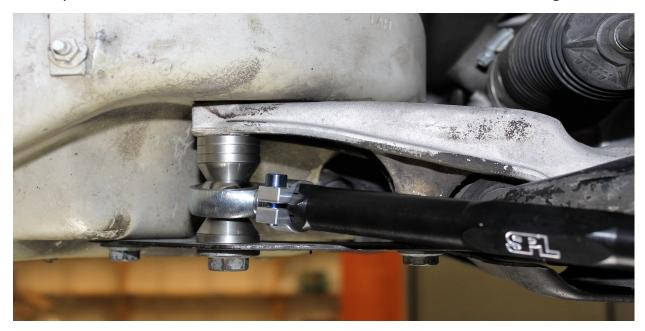
The picture above illustrates washers being used on the caster arm to account for anti dive on the front of the car by lowering the pivot point of the arm shown. Anti squat at the rear of the car is the same principle, except the spacers are placed below the pivot point of the arm for anti squat.
