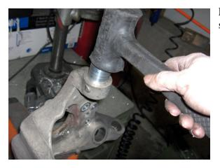
Lightly tap new bushing in place to start, making sure bushing is square against the bore.
