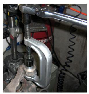
Press out stock bushing using appropriate bushing press and driver.
