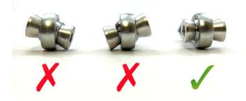
The advantage of the hybrid adjuster is that you can easily keep the rod end bearing centered during and after alignment. Make sure to keep the bearing centered as shown.
