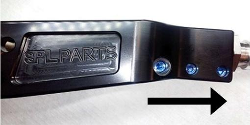
*Tighten Blue Anodized Titanium Head Cap Screws starting from the "SPL Parts" logo, working towards the FK Rod End*
