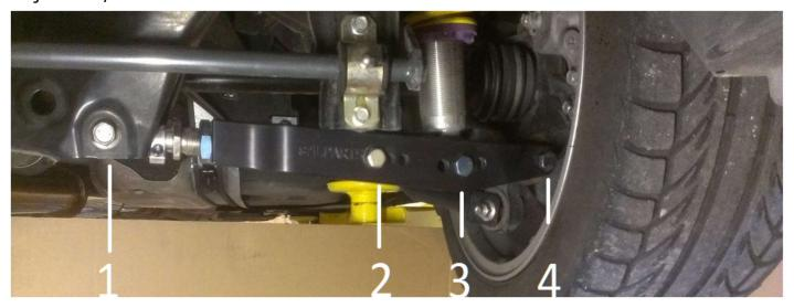
Torque Specs: Bolts 1,3, and 4 – 59 ft. lbs. Bolt 2 – 25 ft. lbs.
