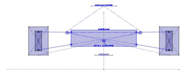
If we are to compare the two subframe positions with the car at the same ride height in both cases, raising the subframe will raise the roll center.
