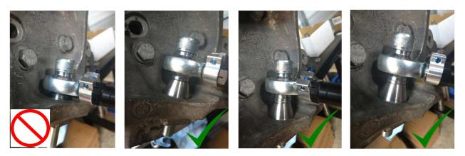
5. The shank (11) is a ½ inch Allen head. Tighten the nut at the top to 110 **ft-lbs**. (Make sure to lubricate the threads; motor oil is fine.) Once tight, check for binding or any problems by moving the suspension through its full travel and moving the wheel lock to lock while doing so. Ensure that the spherical bearing does not bind (the edge of the ball bearing hitting or close to hitting the housing) under any of the above situations and there is no interference between suspension arms.
