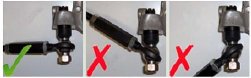
3. Tighten down the 5/8-18 Jam Nut (9) on each end of the Tie Rod End.
