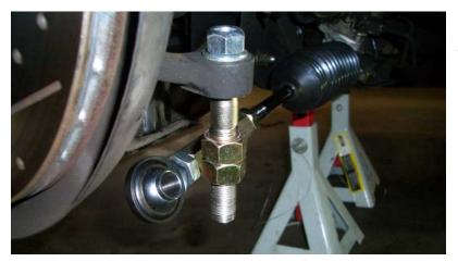
Use 2 supplied 5/8" regular (non-locking) nuts, jam 2 nuts together to help hold the shank.
