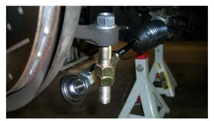
Use 2 supplied gold colored nuts, jam 2 nuts together to help hold the shank. Torque nut on top of knuckle to 40 ft-lbs. DO NOT USE IMPACT GUN OR OVERTORQUE otherwise strength of tie rod end will be severely compromised.
