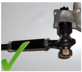
Note that the inner tie rod end can rotate freely, so the picture on left is not binding even though the edge of the ball is touching the housing. If uncertain, try rotating the inner tie rod by using a wrench on the hex part of the inner tie rod:
