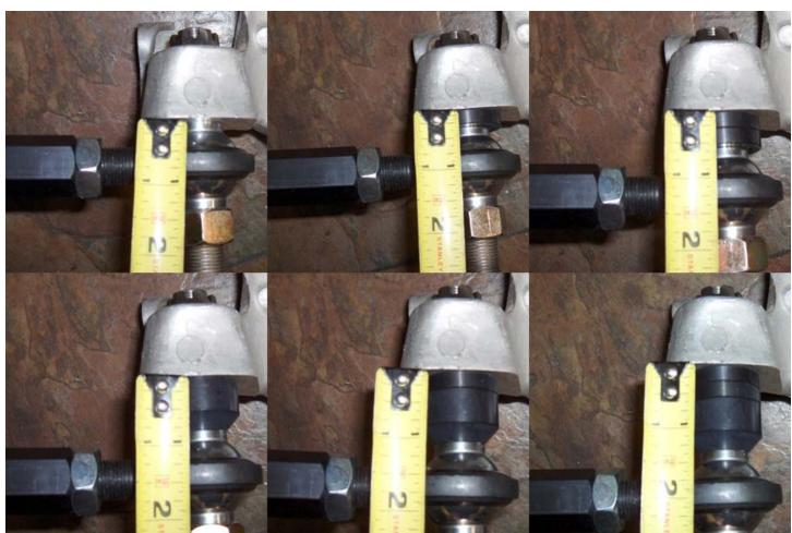
For most installations, we recommend using 3<sup>rd</sup> setting (2 adjustment spacer, no misalignment spacer).
