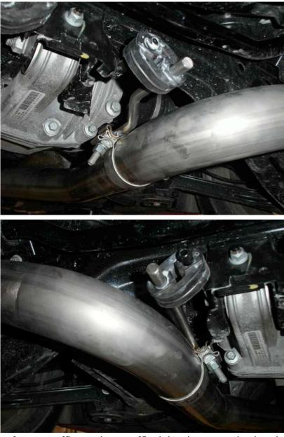
25. Take factory mufflers and cut muffler inlet pipes removing just the flared pieces and deburr. See picture of cutoff flared piece below.
