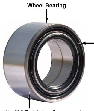
Do not allow Loctite to get into Bearing.
