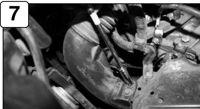
With a 10mm socket or wrench remove both bolts securing the ram air duct to the vehicle
