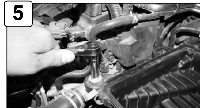
Using 10mm socket or wrench, remove the lower intake box's mounting bolt.
