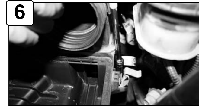
Using a 10mm socket or wrench, remove the mounting bolt on the back of the lower intake box.
