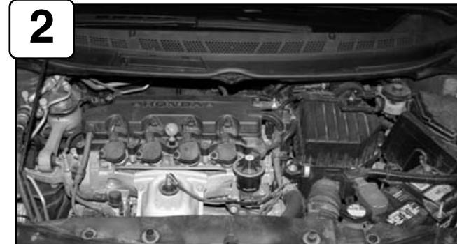
Complete stock intake. Please disconnect battery terminals before installation. Be sure to have your radio security code (if applicable) in order to access your previous settings. Remove the battery and battery tray before install.
