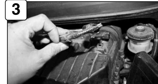
Unplug the MAF sensor harness.
