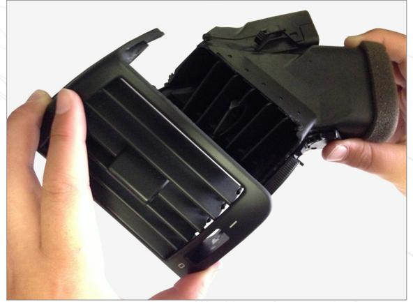
**2** Bend down and forward to break lower bonds and unclip clips.
