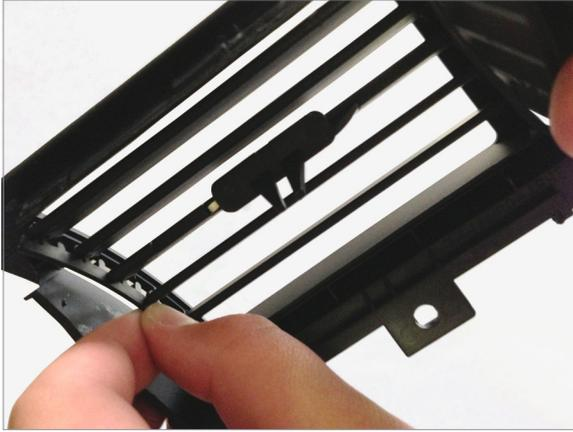
**3** Remove bottom two vent slats from the vent slat keeper.
