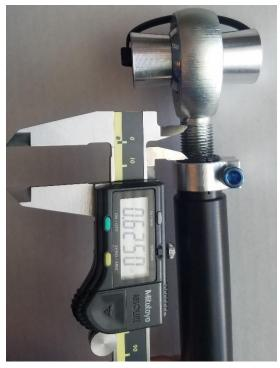
Note the thread engagement on the rod end should not exceed the measurement pictured on the right (0.625''). For the Clevis (1) end, there can be up to (0.625'') of thread exposed.
