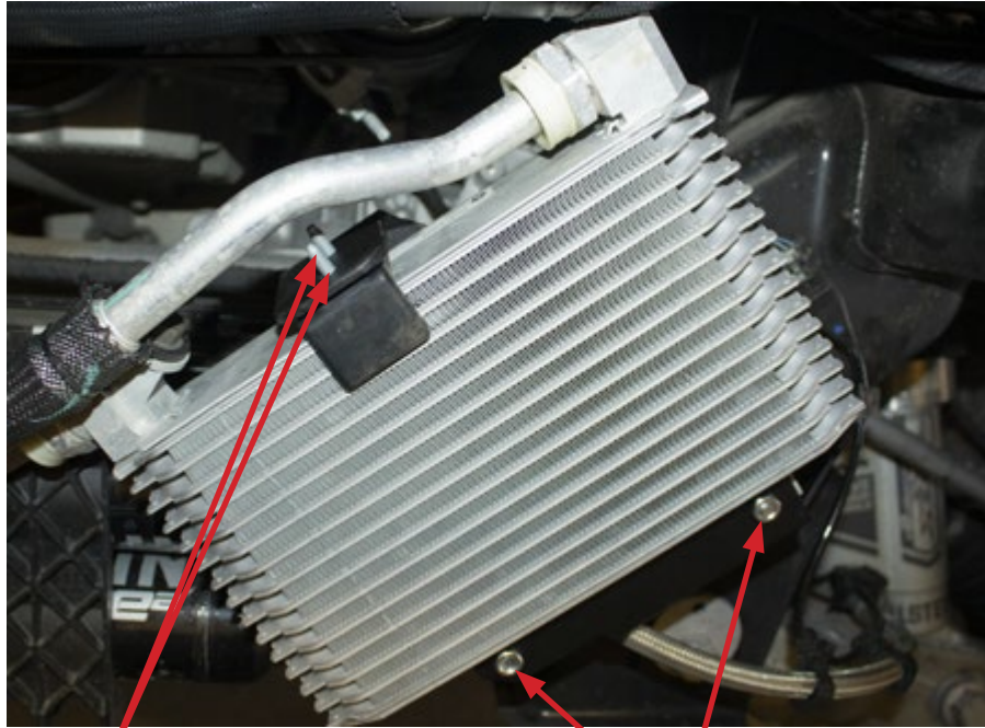
Re-install 2 (10mm) bolts
