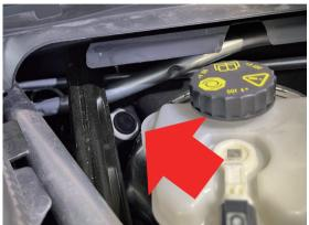
▶ Thread Solenoid Wire from Engine bay into cabin
