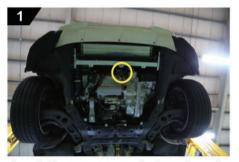
► Locate the vacuum source between the radiator and engine
