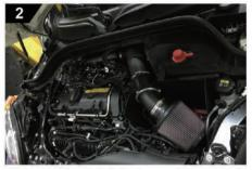
Remove the air intake for easier access to wiring
