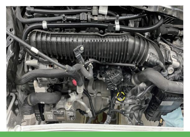
Locate Vacuum source from the brake servo unit
