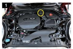
Remove the engine cover to reveal connect-ing location
