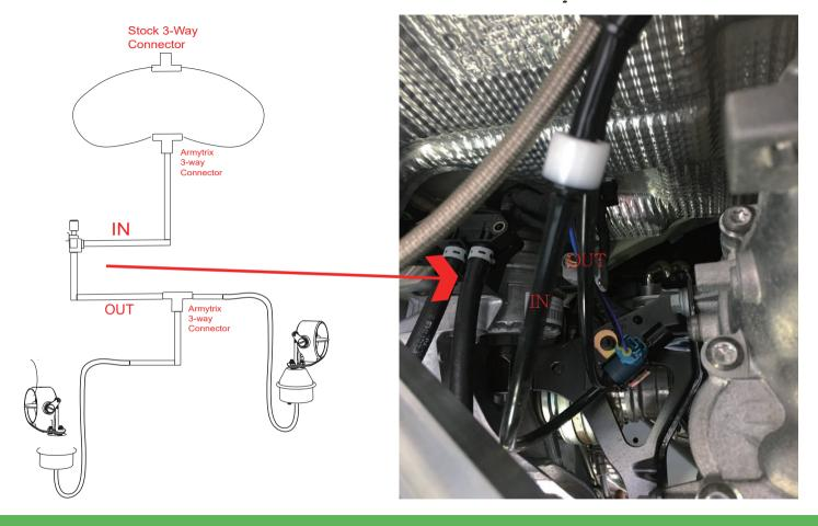
A closer look at where the vacuum source is linked after the 3-way connector is connected
