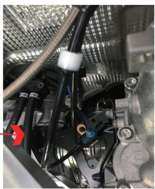
▶ Locate the Solenoid Valve as indicated
