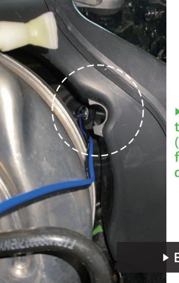
▶ It's recommended to use tools to drag cable directly into cabin (For example, threading iron wire from cabin into engine bay and drag cable into cabin)
