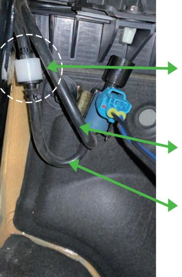
The white end of one-way valve should point to vacuum source
