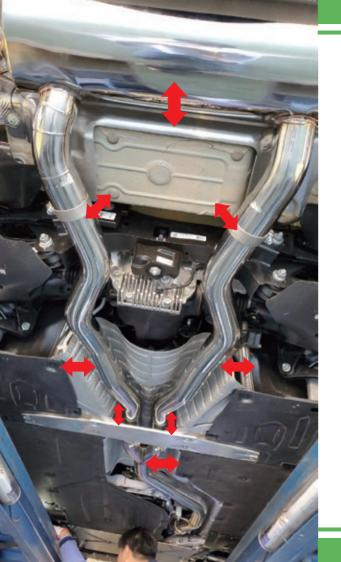
► To prevent damage caused by exhaust thermal expansion / contraction, please make sure leaving at least 1.5-2cm of gap between exhaust system and car body during installation.
