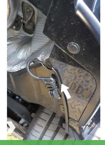
► Connect EV motor delete cap with OEM electric valve plug.
