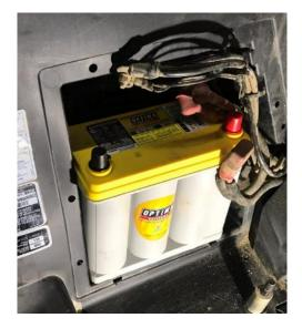
c) Remove the stock rubber terminal cover over the Positive cable, feed the new provided terminal covers onto both the negative and positive wires.
