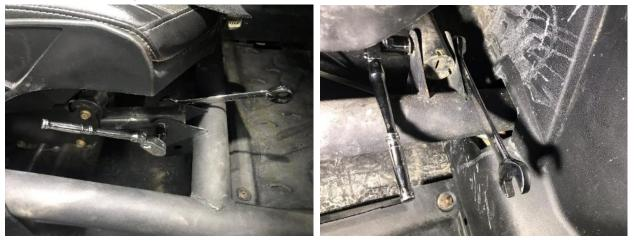
e) Remove the Seat from the car, the seat belts will come out with the seat.
