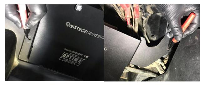
c) Remove the Battery plate and then drill both holes at the marked locations using an 11/32" Drill Bit and Power Drill
