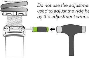
Do not use the adjustment wrench to lock the lower mount, it is only used to adjust the ride height. If the lower locking collar is tightened by the adjustment wrench, it MAY COME LOOSE.
