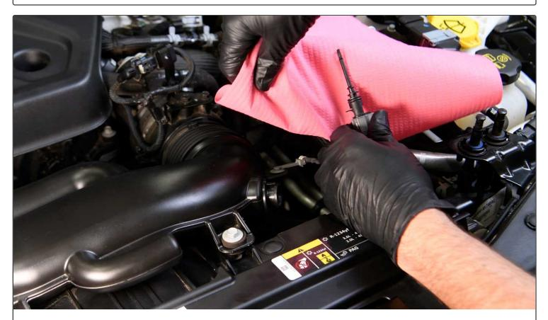
2. Unhook the two clips securing the IAT harness to the factory
