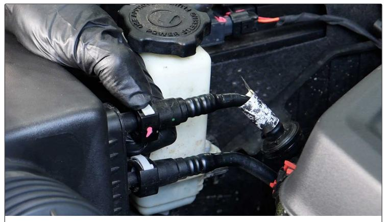
6. Remove the two plastic lines from the air filter housing by
