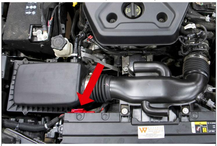
NOTE: Before removing the entire assembly, take note of the sensor connection highlighted in the photo.
