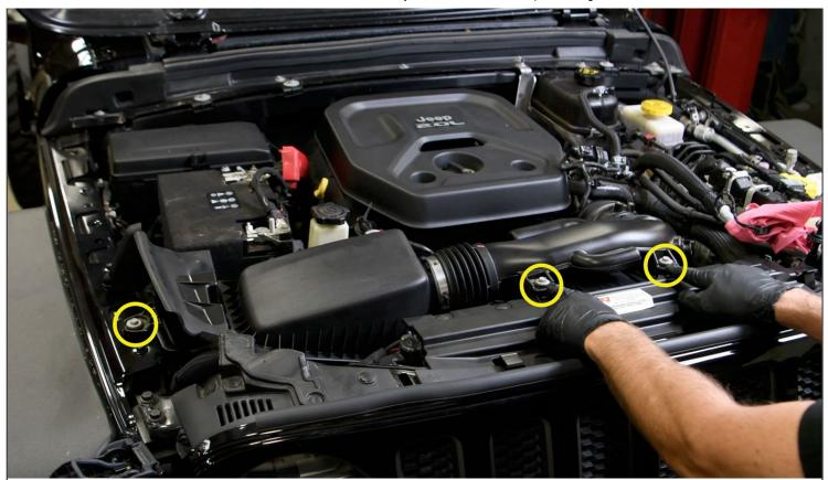
5. Using a 10mm socket, remove the three bolts holding the OEM intake system.
