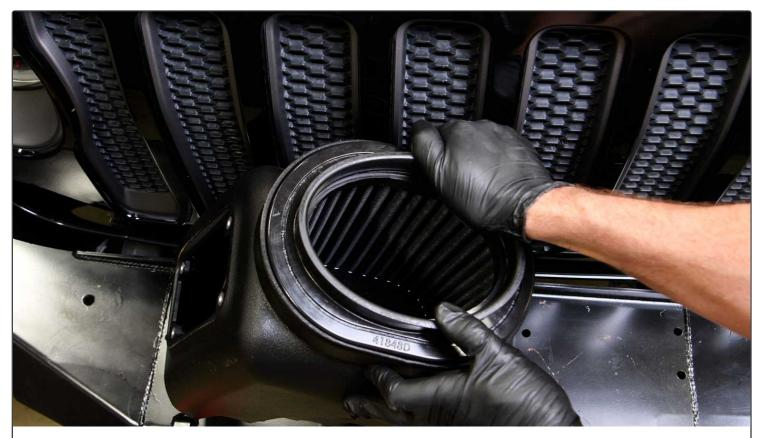
12. Install the Banks air filter into the Banks airbox and make sure the arrow on the filter is on top.
