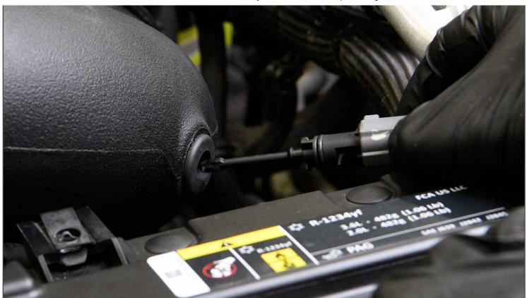
23. Insert the IAT sensor into the rubber grommet.
