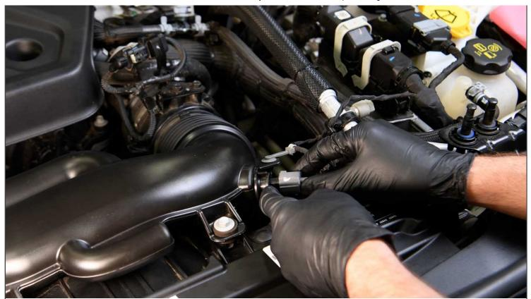
1. Remove the IAT sensor. Pull the locking clip towards you and twist counter-clockwise about 45 degrees until it stops rotating.
