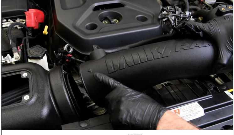
21. Install the Banks intake tube by first inserting the large end into the filter and then the smaller end into the OEM turbo inlet duct. Align the duct to the indent on the tube. Align the arrows on the tube and filter. Tighten both clamps.
