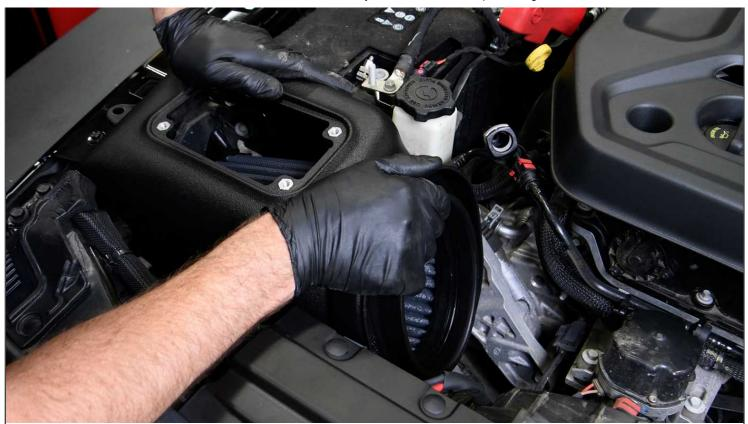
13. Install the Banks Ram-Air box into the engine bay by pressing down until it pops into the rubber grommets.
