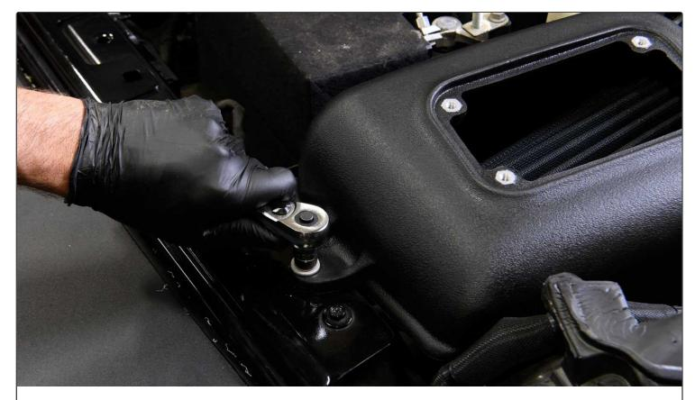
14. Secure the Banks Ram-Air box to the sidewall by using the
