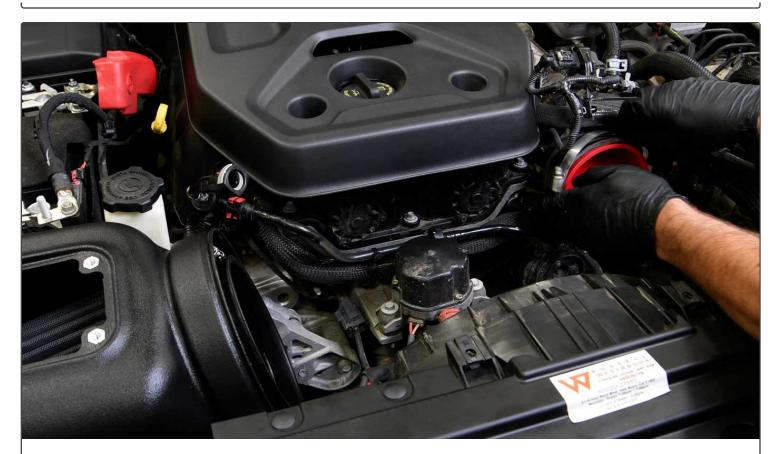
20. Place the smaller hose clamp over the factory turbo inlet duct.
