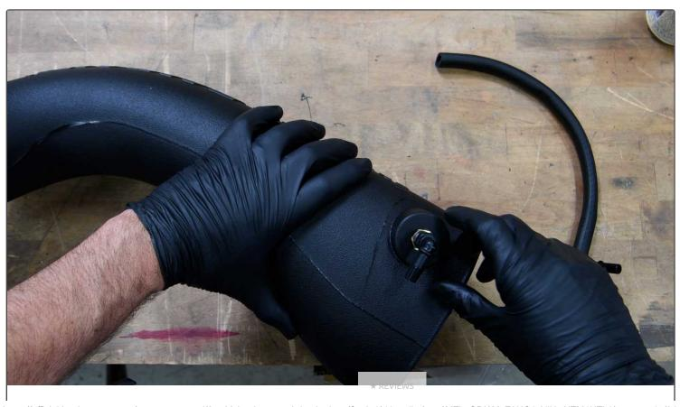
16. Take the supplied plastic barbed hose elbow and thread it into the Banks intake tube. The barbed end should be at the 6 o'clock position.
