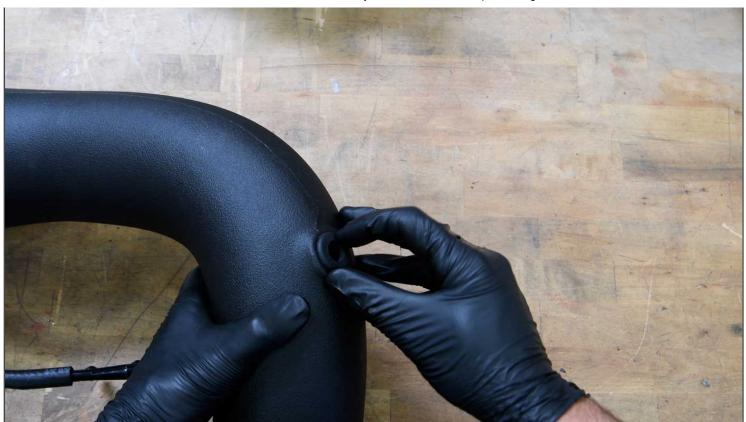
18. Install the rubber grommet for the IAT sensor onto the intake tube.
