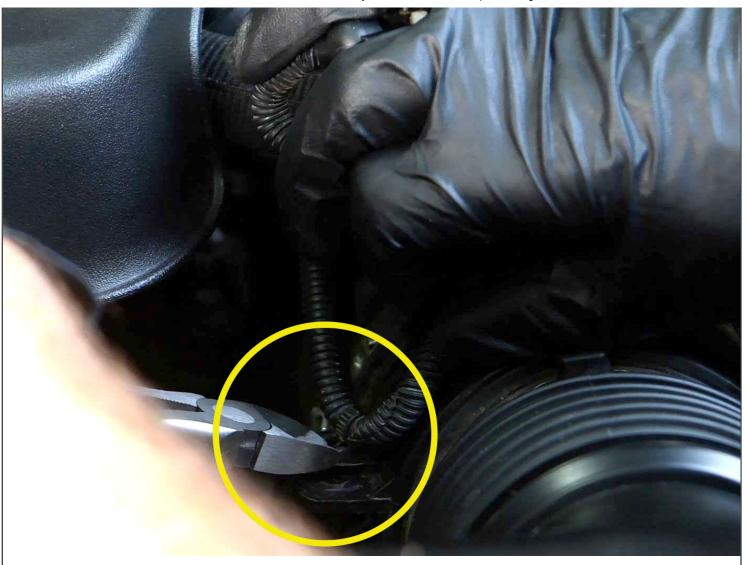
4. Cut off the plastic tie that holds the wiring harness to the OEM intake tube.
