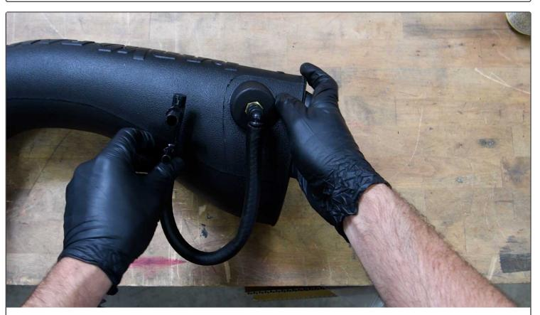
17. Once the fitting is installed, connect the open end of the hose to the fitting. Make sure you can make a loop with the hose, as shown.
