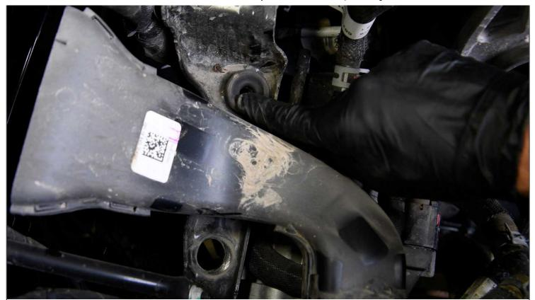
NOTE: It's very important that you install the grommets into the engine bay and NOT onto the Banks airbox.
