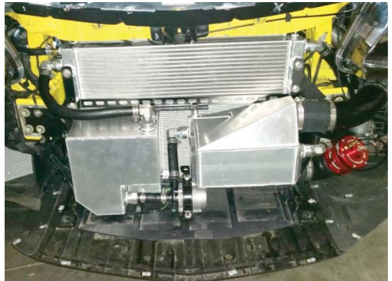
Coolant Plumbing Complete
