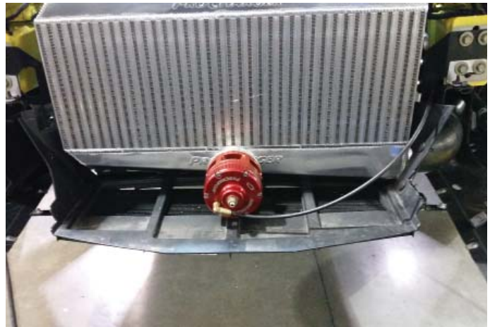
Modified Air Shroud Installed
