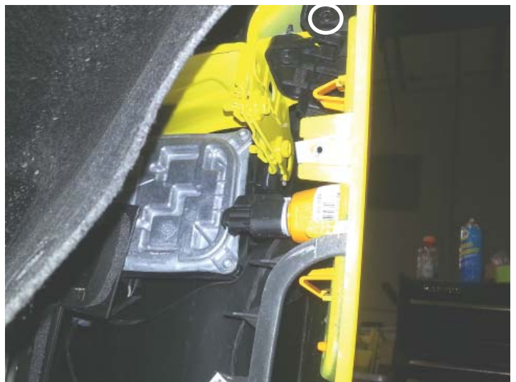
Screw Behind Wheel Liner
