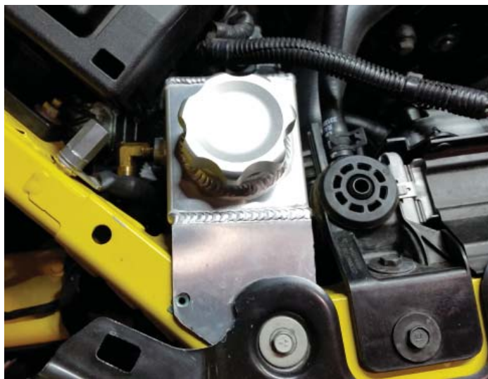
Fill Tank Installed
