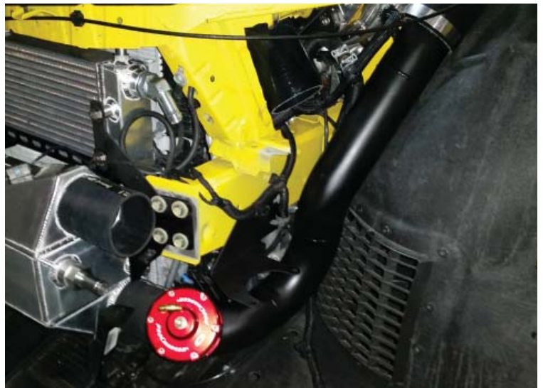
Blower Outlet Tube Installed
