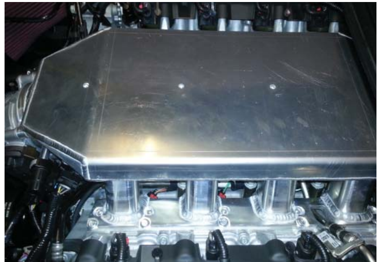
Intake Manifold Install
