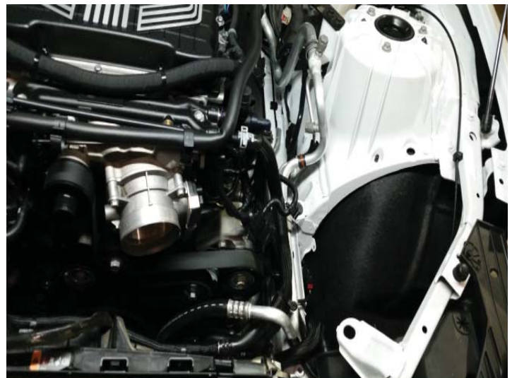
Air Inlet Removed
