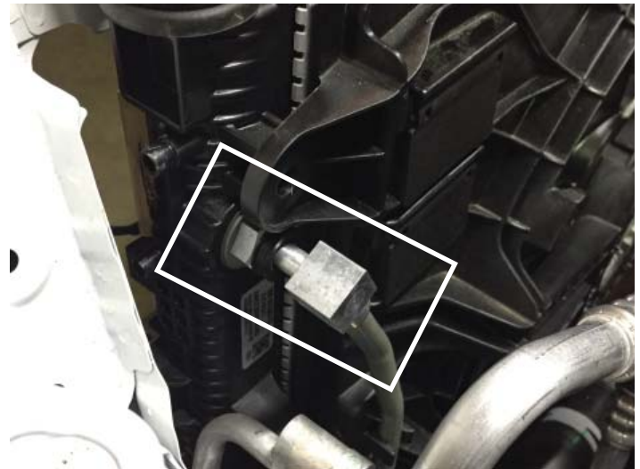
Transmission cooler line.
