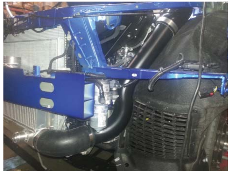
Lower Intercooler Connection
