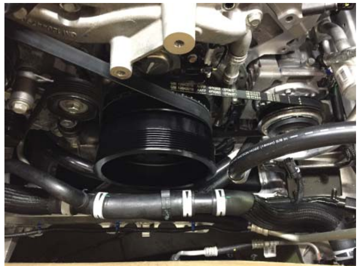
Crank Pulley Installed
