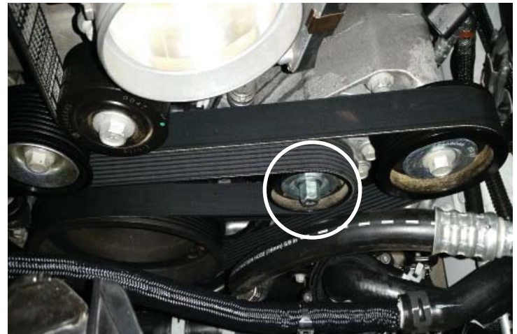
Supercharger Belt Tensioner
