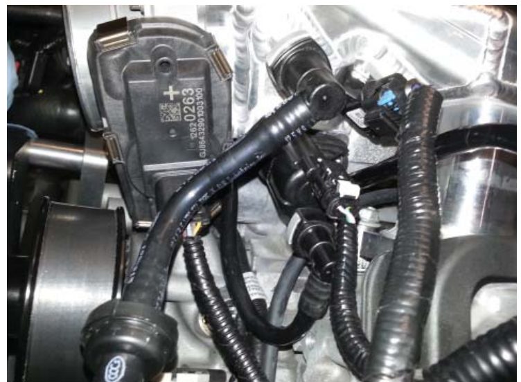
MAP, EVAP and PCV Lines Connected
