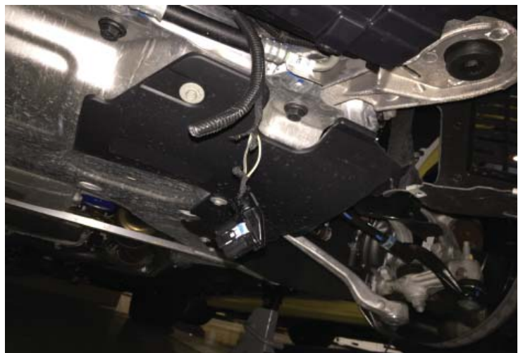
Intercooler Pump Wiring
