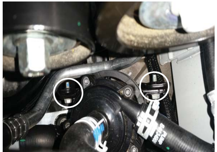
Intercooler Pump Bolts
