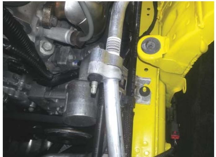
Factory A/C Line Bracket
