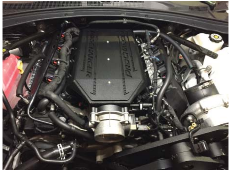
Intake Manifold Installed
