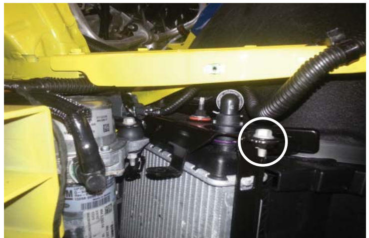
Aux. Heat Exchanger Bracket Bolts
