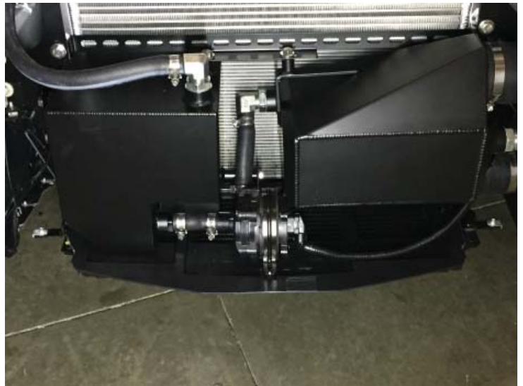
Modified Air Shroud Installed
