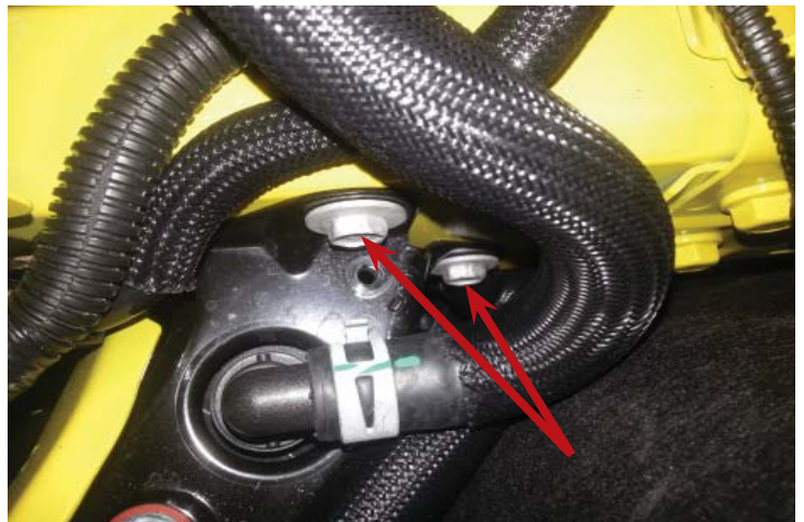
Upper Aux. Heat Exchanger Bolts
