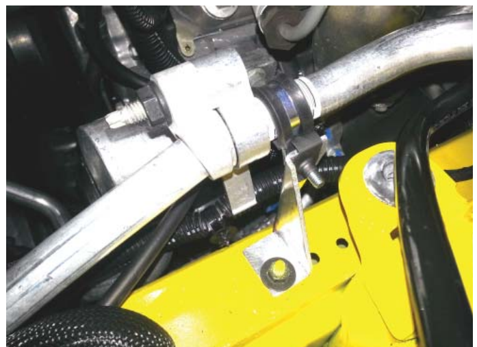
Factory A/C Line Bracket
