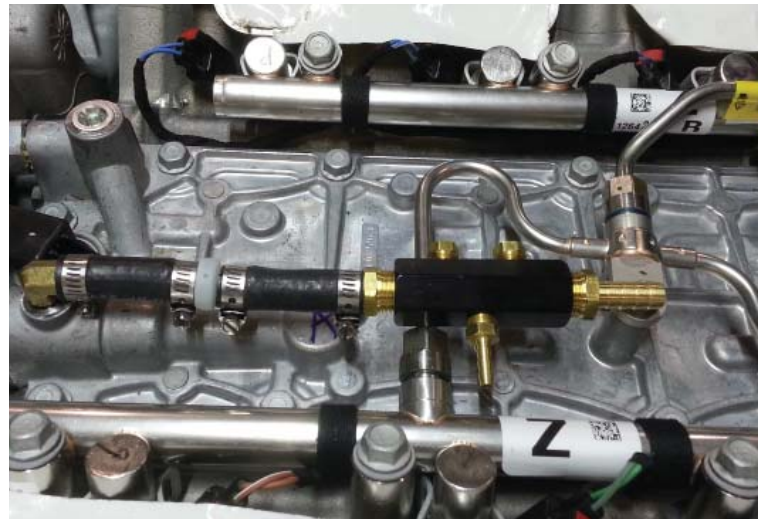
Vacuum Manifold Installed
