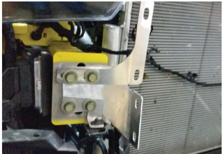
Brackets Mounted (Right Side)
