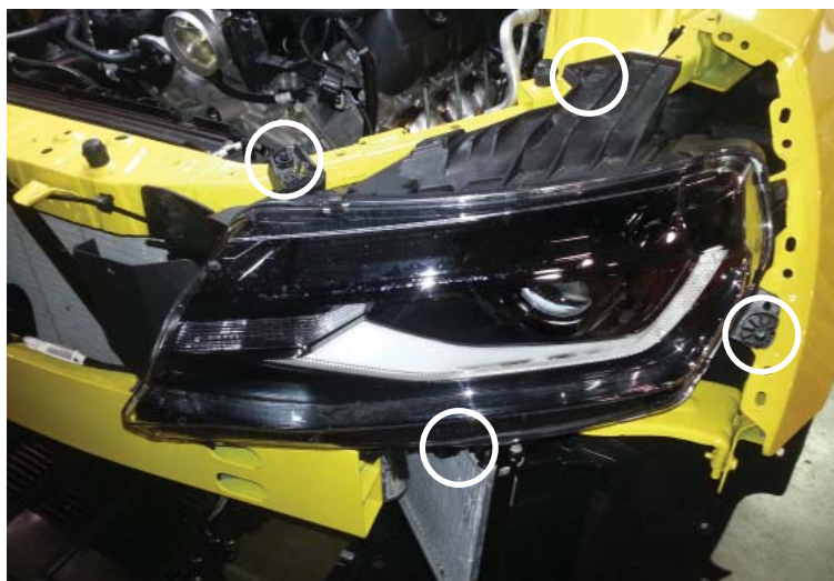
Remove Headlight Screws
