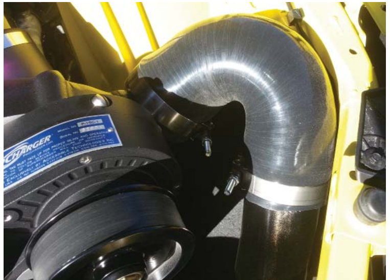
Blower Discharge Tube Installed
