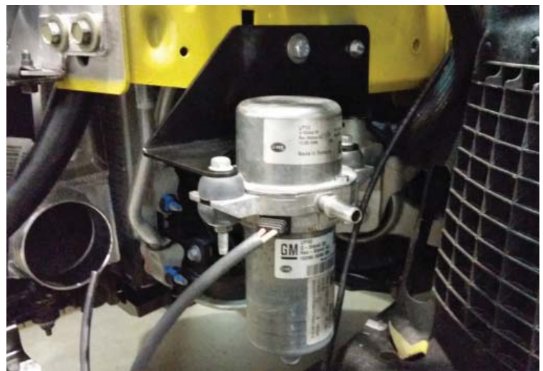
Brake Pump Relocated
