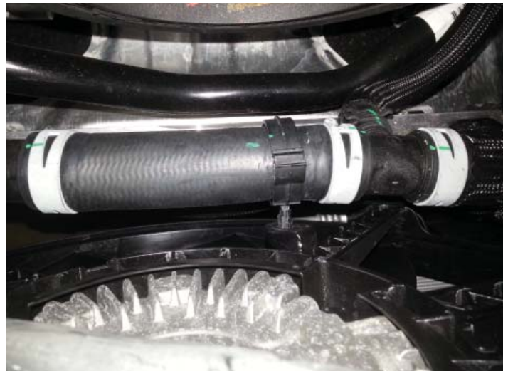
Disconnect Radiator Hose From Fan
