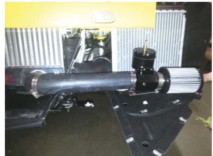
Surge Valve Installed
