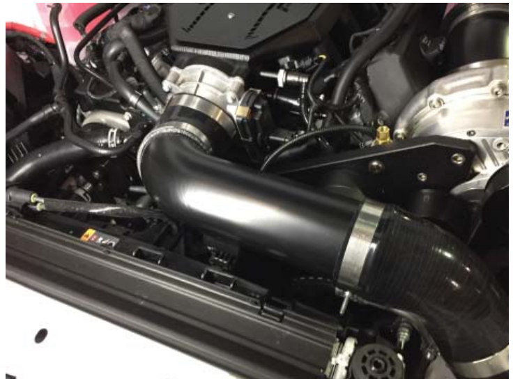
MAF Tube Routing
