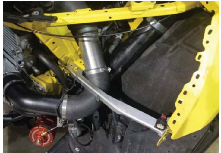
Install New Fender Brace
