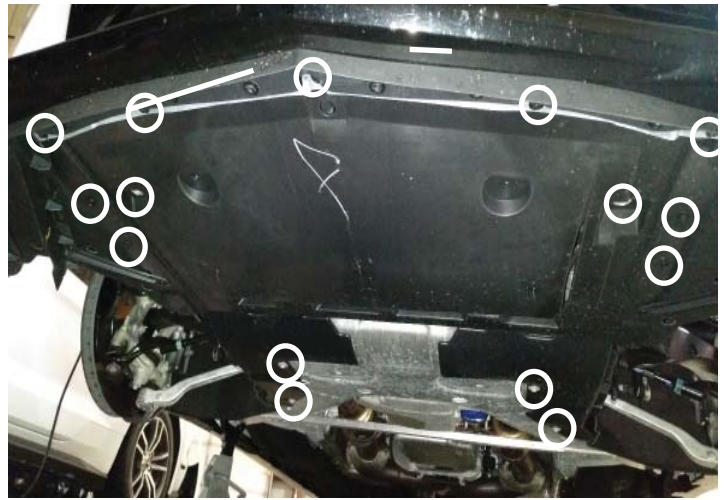
Plastic Splash Panel Screws and Bolts
