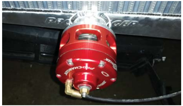
Race Valve Installed
