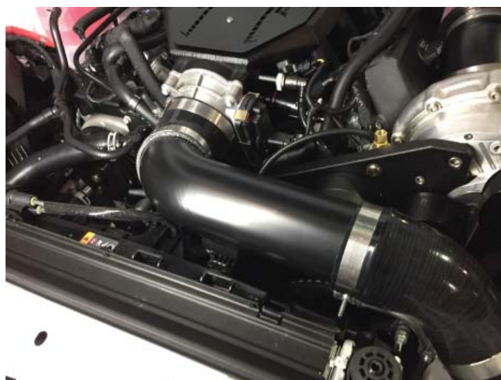
MAF Tube Routing
