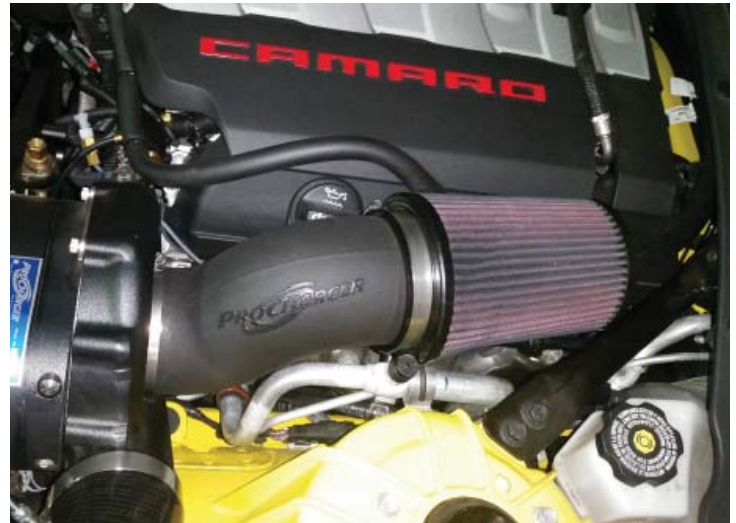
Air Inlet Installed
