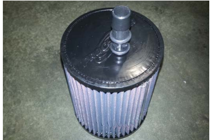
Plastic Fitting Installed in Air Filter
