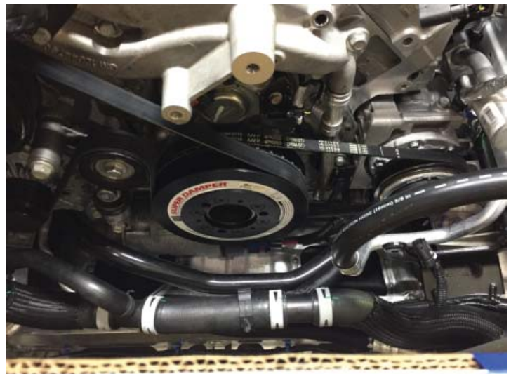
ATI Balancer Installed
