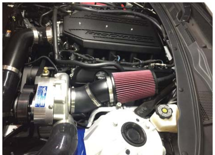
F1A-94 Air Inlet Installed
