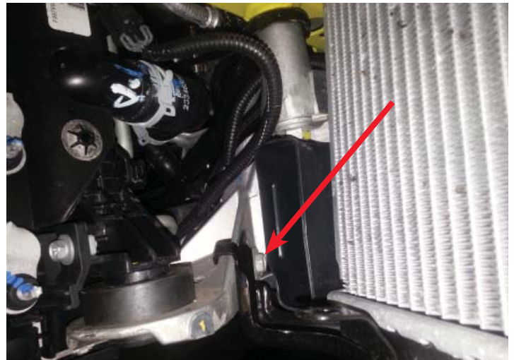
Lower Aux. Heat Exchanger Bracket Bolt
