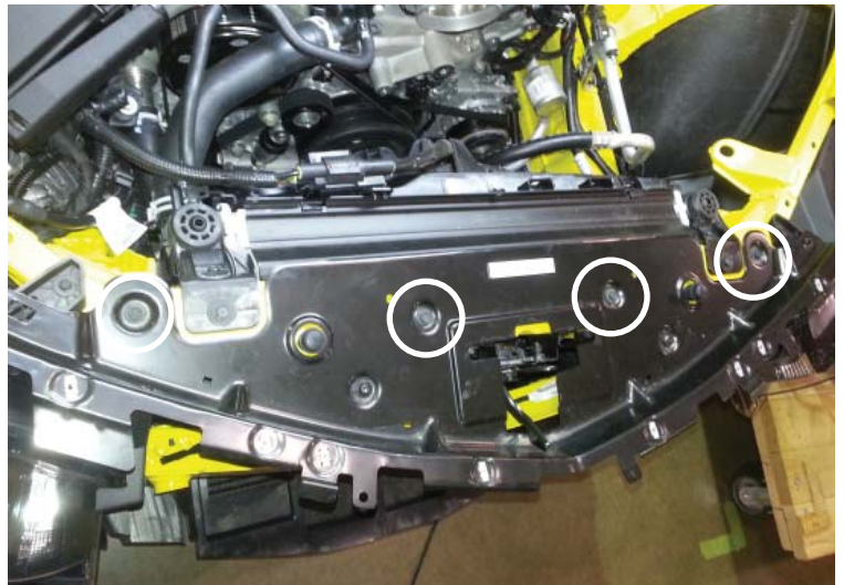
Remove Radiator Cover Bolts
