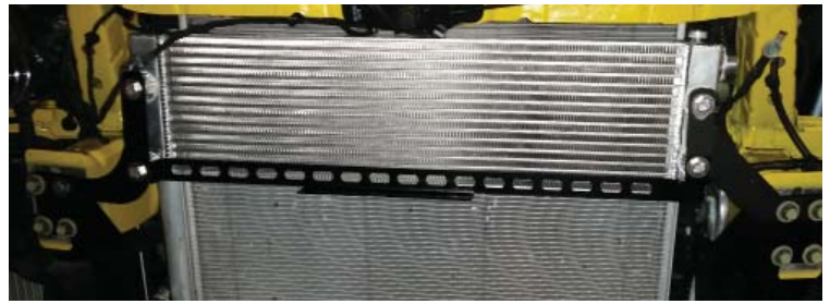
Heat Exchanger Mounted
