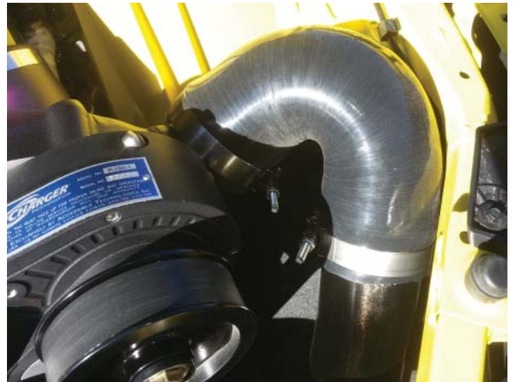
Blower Discharge Tube Installed
