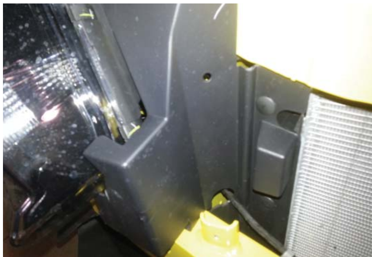
Plastic Radiator Cover (Passenger's)
