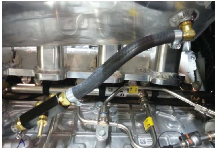
Vacuum Manifold Connected to Intake
