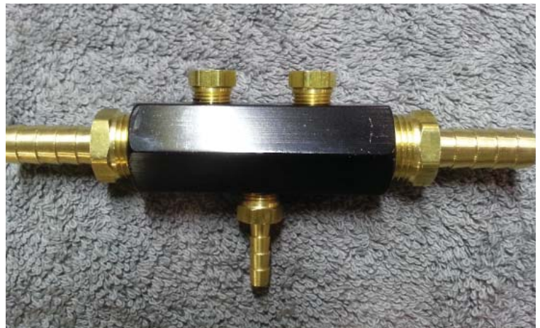
Vacuum Manifold Assembled
