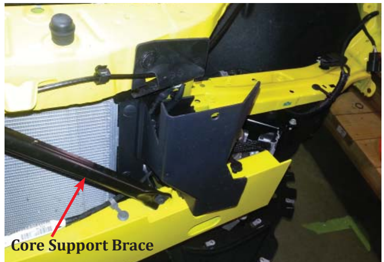
Remove Plastic Covers (Driver's Side)
