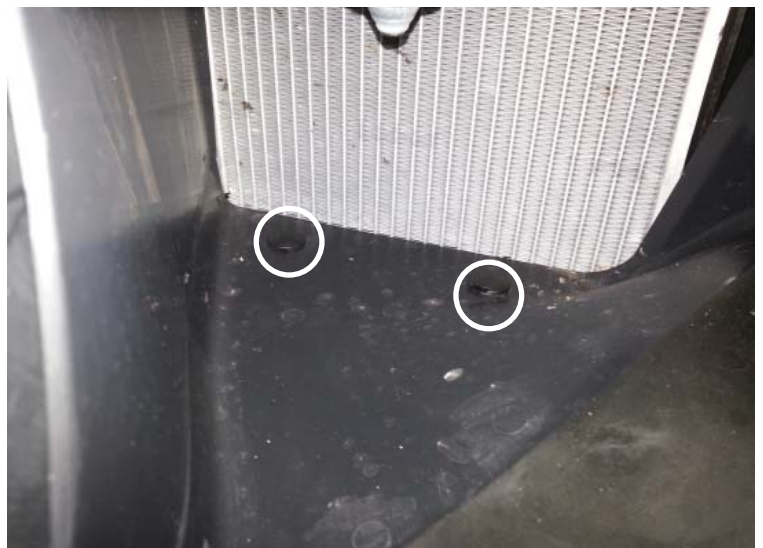
Radiator Scoop Push Clips
