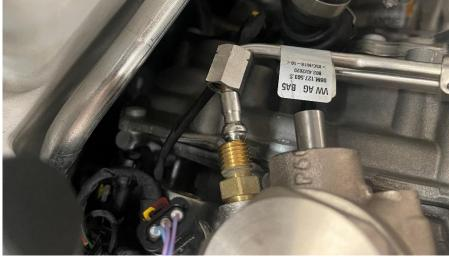
**Step 13** Using an M10 triple-square, remove the hardware securing the fuel pimp housing to the engine.
