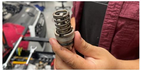
**Step 22** Place the 034 spring retaining washer over the spring.
