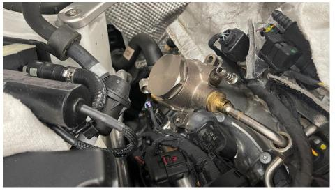
**Step 28** Using an M10 triple-square, reinstall the hardware securing the fuel pump housing to the engine.
