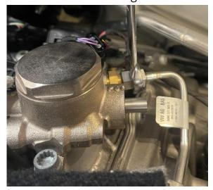
**Step 30** Using a T30 Torx, reinstall the hardware for the hard fuel line bracket.
