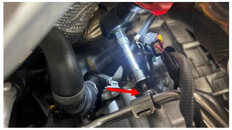
**Step 11** Using a 14mm wrench, loosen the hard line from the back of the housing.
