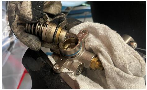
**Step 18** Remove the piston sleeve from the spring assembly.
