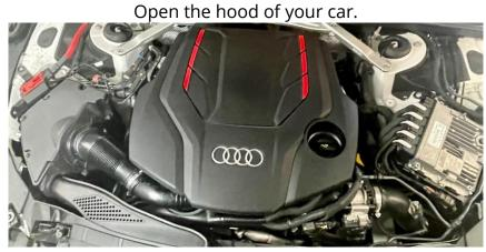
**Step 2** Remove the engine cover by pulling it up.
