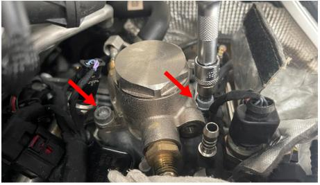
**Step 14** Remove the fuel pump housing.
