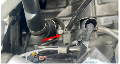
**Step 32** Using a 27mm wrench, reinstall the pressure sensor fitting at the back of the housing.
