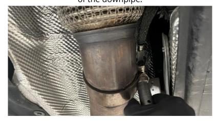
**Step 12** Slide the stock downpipe off of the mounting brace and remove it from under the car.
