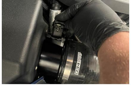
**Step 21** Reconnect the intake hose to the MAF housing and secure it with the hose clamp.
