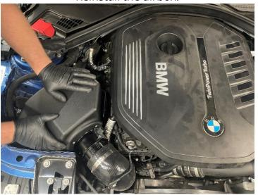
**Step 20** Reconnect the MAF sensor connector.
