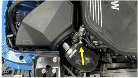
**Step 4** Remove the airbox by firmly pulling up.
