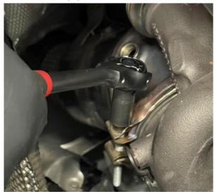
**Step 8** Using a 13mm socket, remove the nuts from the downpipe mounting brace.
