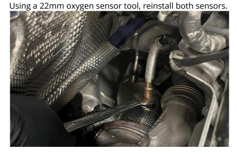
**Step 17** Reconnect the oxygen sensor connector.
