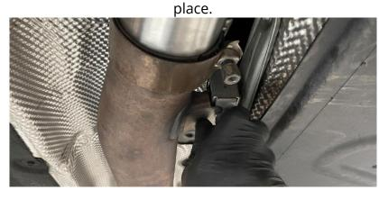
Step 24 Using a 13mm socket, secure the exhaust clamp back into
