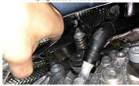
**Step 12**Using a 13mm wrench, tighten the rear exhaust clamps.
