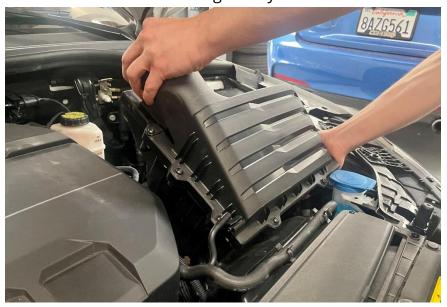
**Step 8**Push the S34 assembly onto the mounting posts.
