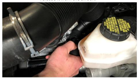
**Step 5** Extract the intake hose from the engine bay.
