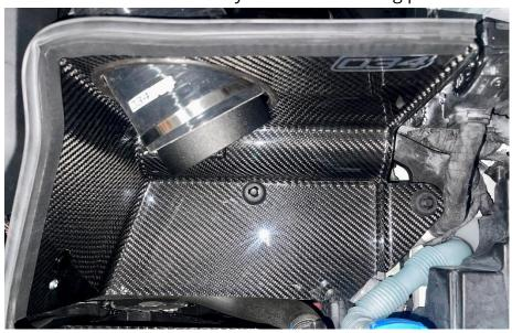
**Step 9**Install the silicone hose onto the turbo inlet.
