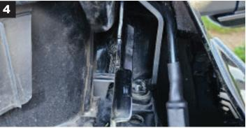
THE DITCH BRACKET NEEDS TO TWIST DOWN INTO PLACE TO CLEAR THE HOOD AND HINGE. ONCE POSITIONED CORRECTLY, THE UPPER TAB & LOWER TAB SHOULD ALIGN WITH THE BOLT HOLES. RE-INSTALL THE FACTORY M8 OEM HEX BOLT.
