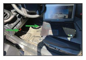
17. Turn the ignition switch to the on position (Engine off). On Tacoma's /
