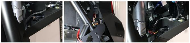
WARNING! Make sure to keep the harness away from any hot or moving parts
