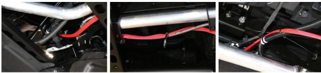
Cross over to the passenger side, secure harness to brake line and battery cable, continue to the front.
