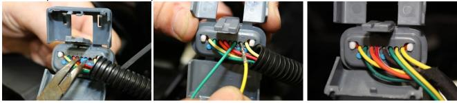
9. Close Cover – Run ATS wires alongside the OEM harness and snap shut, re-install plastic locking cover and plug back in.
