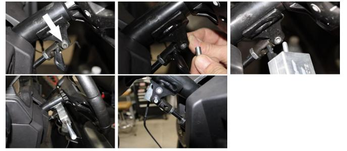
5. Install the Horn/Hazard Switch. Remove 1 of the switch plugs.
