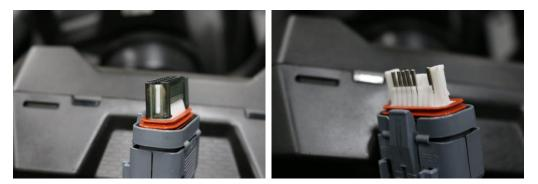
8. Remove Plugs – Using a pair of needle nose pliers remove the plugs from wire port 6 and 7, insert green wire terminal into 6 and yellow wire terminal into port 7.
