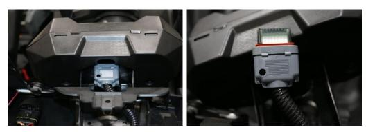
7. Remove Connector Lock – Using a small screwdriver push in on both sides at the white connector shown below and slide lock off
