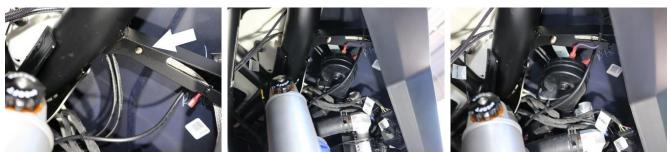
11. Plug the Power Harness into the Control Module. Run the power wire to the Busbar, remove one of the blanks and plug into the Busbar.
