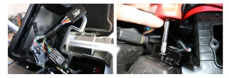
14. Using the provided Cable Tie's secure the harness completely. Reinstall any removed parts.
