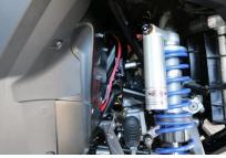
Make sure to run the harness inside of the frame away from the control arm, going through the rubber grommet in the fire wall
