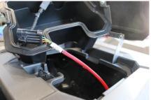
Open the Dash storage and remove the tray, run the harness up into the compartment. Plug into the Control Module. WARNING! Verify that there is clearance where you want to mount the front LED lights before drilling the holes!
