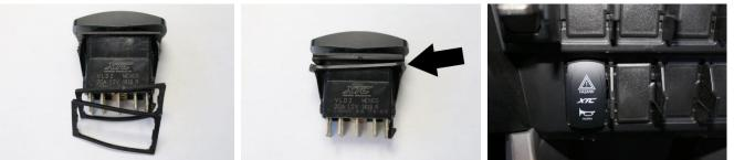
Run Switch Harness–Plug the Switch Harness into the Control Module, run Horn/Hazard connector through the rectangle switch cutout and use included grease on switch terminals then connect Switch and slide into dash. **NOTE:** The switch cut outs are counter sunk, we have supplied 2 switch seals to be used as spacers to keep it raised out of the indent to keep it from getting stuck.
