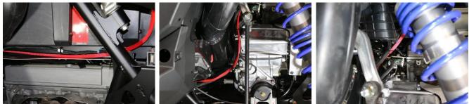
Follow the brake line down the chassis, at the mid-section there is a battery cable going over the drive shaft
