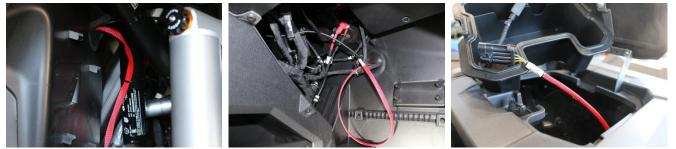
Open the Dash storage and remove the tray, run the harness up into the compartment. Plug into the Control Module. WARNING! Verify that there is clearance where you want to mount the front LED lights before drilling the holes!
