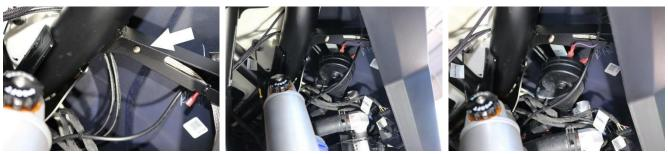
6. Plug the Power Harness into the Control Module. Run the power wire to the Busbar, remove one of the blanks and plug into the Busbar.
