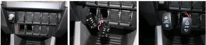
Run Switch Harness–Plug the Switch Harness into the Control Module, run the two connectors through the rectangle switch cutouts and use included grease on the terminals then connect to turn switch and slide switch into dash. **NOTE:** The switch cut outs are counter sunk, we have supplied 4 switch seals (2 for each Switch) to be used as spacers to keep it raised out of the indent to keep it from getting stuck.
