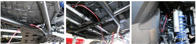
Make sure to run the harness inside of the frame away from the control arm, going through the rubber grommet in the fire wall
