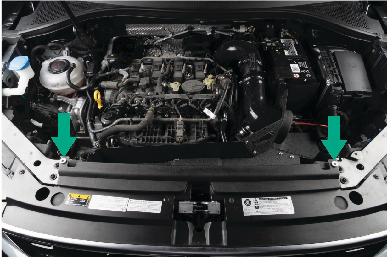
Install two 4mm bolts to secure the scoop to the radiator core support.
