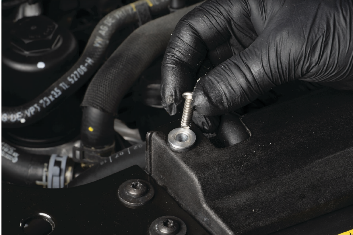
Install two 4mm bolts to secure the scoop to the radiator core support.
