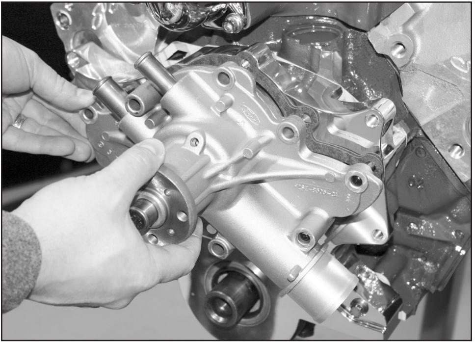
Figure 7: Install Water Pump
