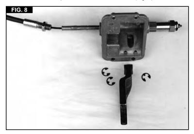
25. Press the button and pull the cable approximately 1" to the full engaged position. Check to see that the stop E-clip is resting against the housing. Note: the CAD housing must be removed from the axle in order to adjust the fork travel. If the E-clip does not contact the housing, thread the cable out until it does.
