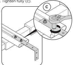
**Mounting Awning - Option B**For Rooftop Rack with Cross Bars (with channels)
