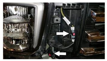
4. Remove the factory side brackets. There will be (3) 15mm bolts on each side.
