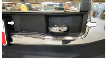
5. Install the bottom mounting brackets. Line the top hole of the bracket over the top hole of the bumper. Reuse some of the bolts and nuts from step #1. (Photo of driver side)
